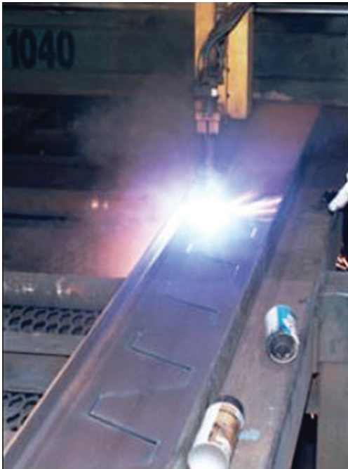
Fig. 1-2. Cutting of a castellated pattern.
