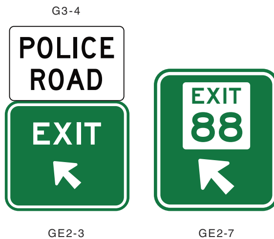
Figure 3.5 — EXIT gore sign (GE2-3) with optional road name sign (G3-4); optional Exit number gore sign (GE2-7)
