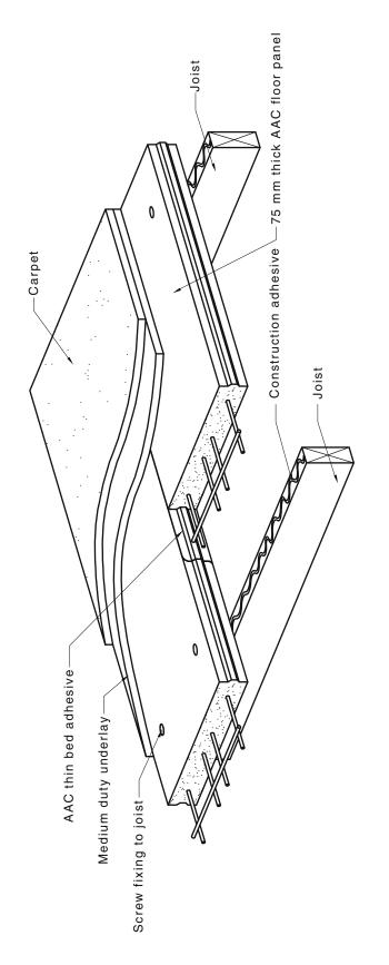
FIGURE 6.3(A) (in part) 75 mm THICK REINFORCED AAC FLOOR WITH CARPET
