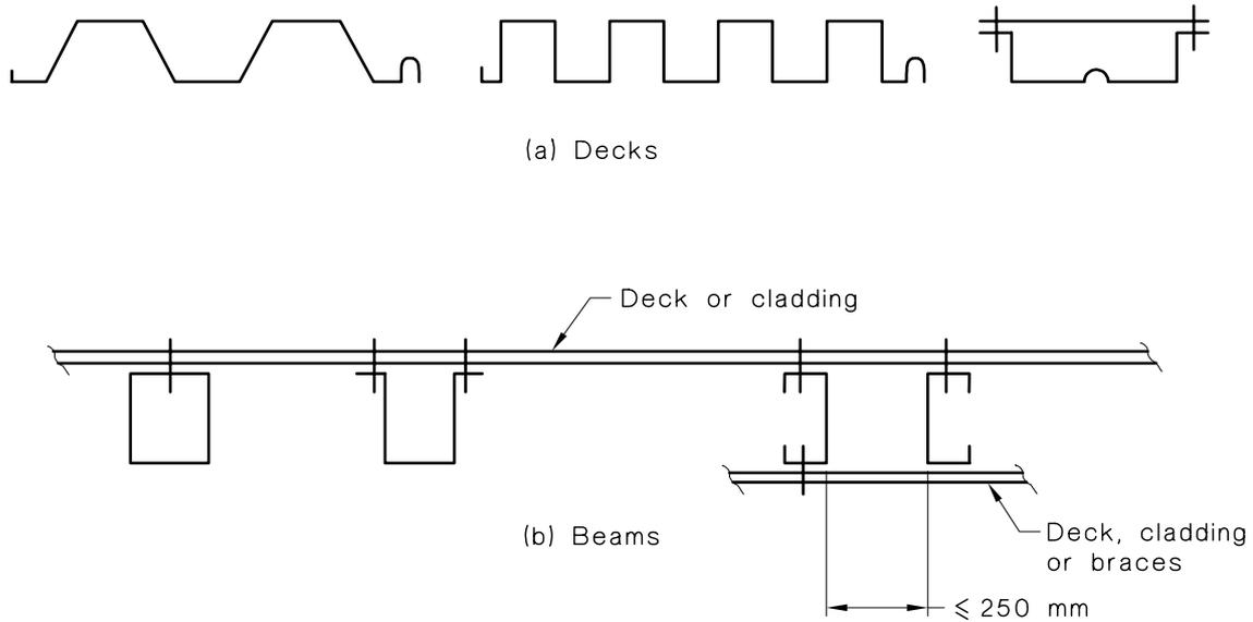
FIGURE C3.3.7(3) SECTIONS USED FOR EXCEPTION OF CLAUSE 3.3.7(a) OF THE STANDARD
