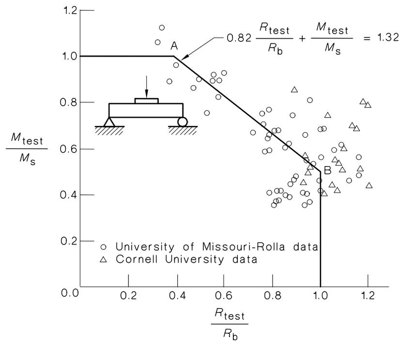
FIGURE C3.3.7(2) INTERACTION BETWEEN WEB CRIPPLING AND BENDING FOR I-BEAMS HAVING UNREINFORCED WEBS
