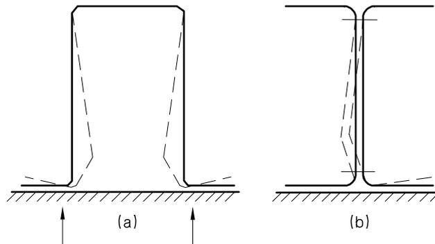
FIGURE C3.3.6(1) WEB CRIPPLING OF COLD-FORMED STEEL BEAMS
