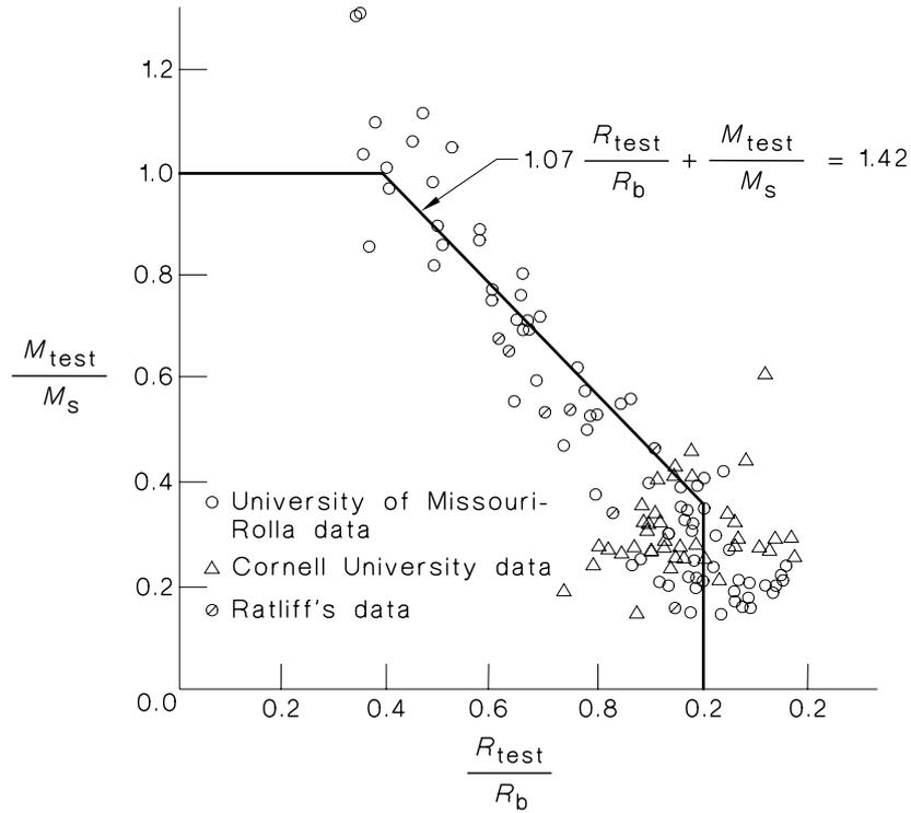
FIGURE C3.3.7(1) GRAPHIC PRESENTATION FOR WEB CRIPPLING AND COMBINED WEB CRIPPLING AND BENDING FOR SINGLE UNREINFORCED WEBS
