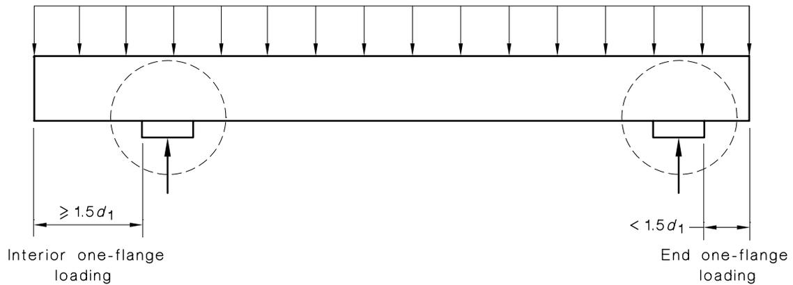
(a) One interior and one end one-flange loading
