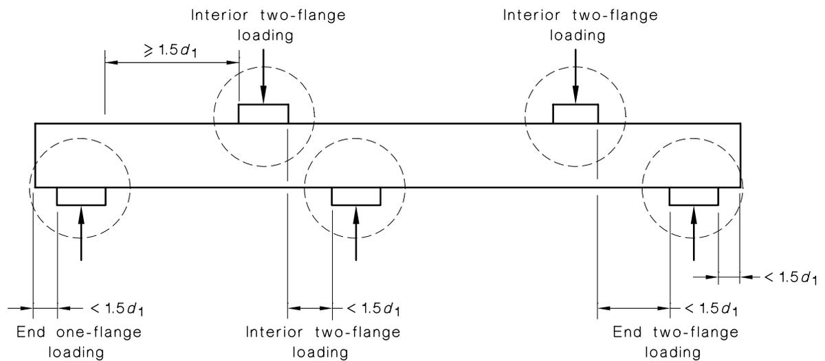
(b) Three interior two-flange, one end one-flange and one end two-flange loading
