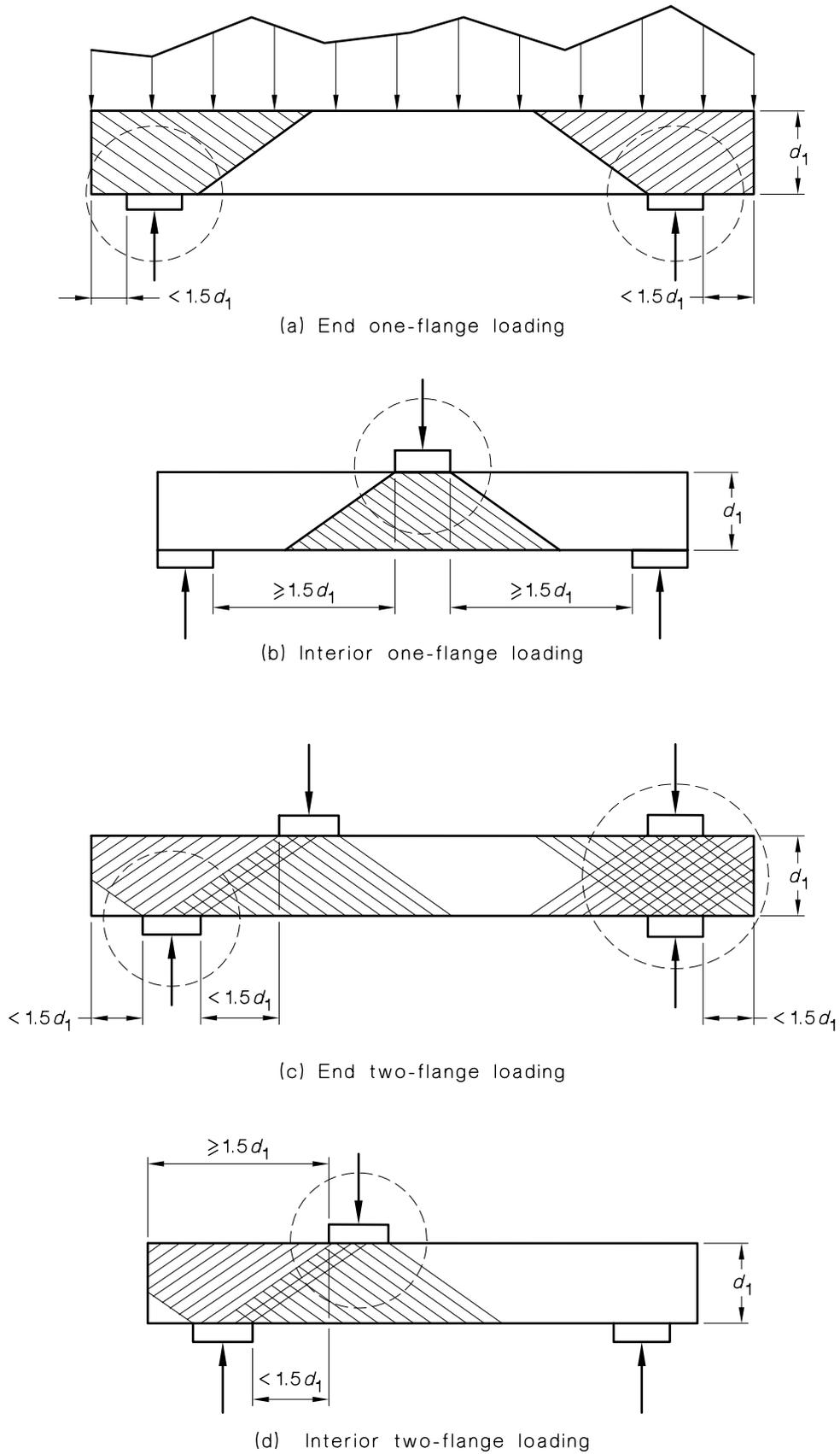
FIGURE C3.3.6(4) ASSUMED DISTRIBUTION OF REACTION OR LOAD
