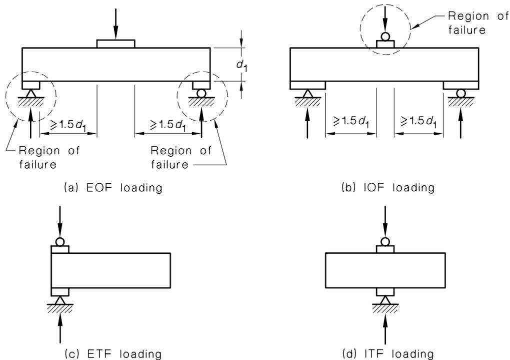
FIGURE C3.3.6(2) LOADING CONDITIONS FOR WEB CRIPPLING TESTS
