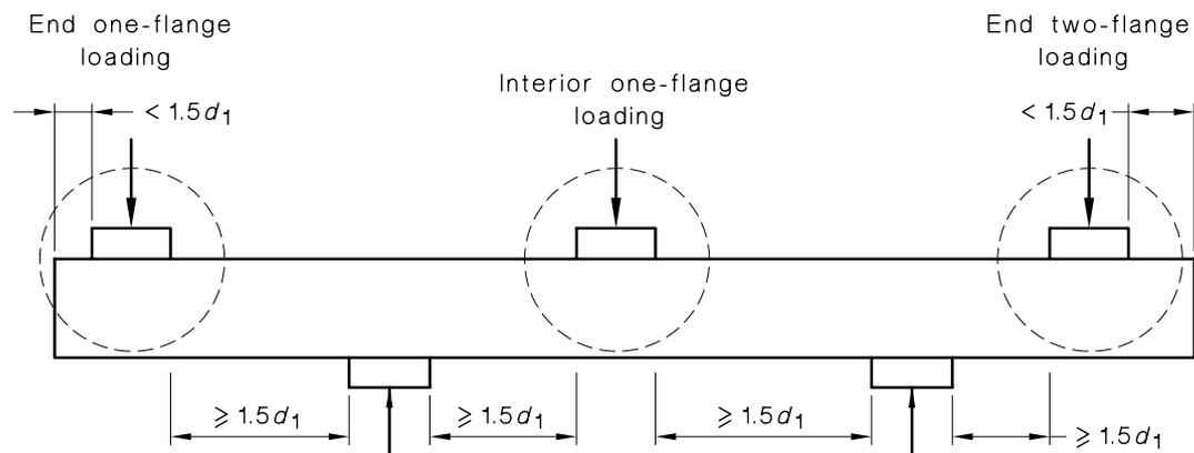
(c) One interior one-flange, one end one-flange and one end two-flange loading
