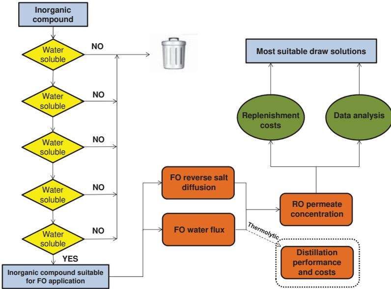
Figure 14.21. Flow chart for draw solution selection
