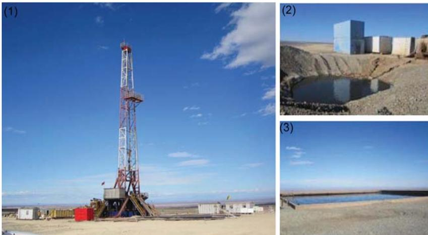
Figure 15.2. Photos of one typical shale gas exploitation site in west China. (1) Shale gas exploitation well pad; (2) domestic wastewater; (3) wastewater storage
