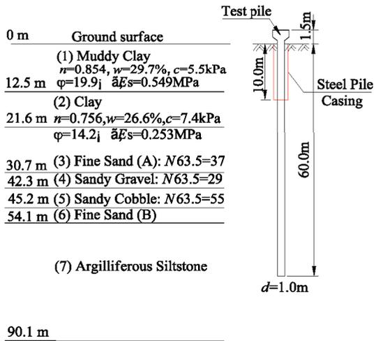
**Fig. 1. Soil profile around the test pile.**
