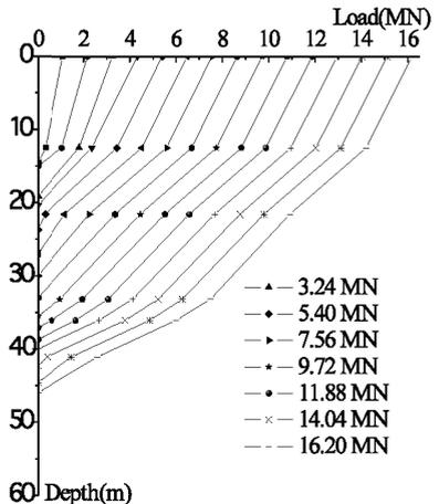
**Fig. 4. Pile shaft axial force distribution.**
