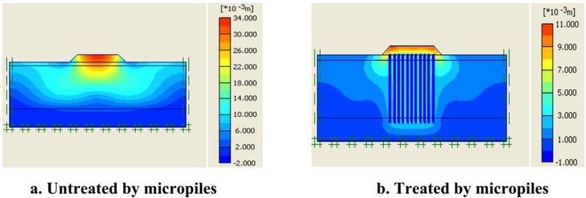
**FIG. 2. FEM plot of extreme total displacement.**
