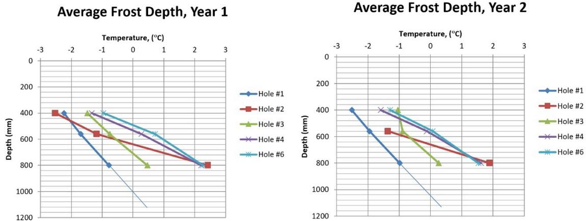
Figure 8. Average thermistor temperatures as a function of depth over the two winters.
