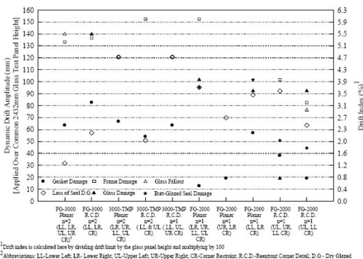
**Figure 11. Summary of test data for all mockups tested.**
