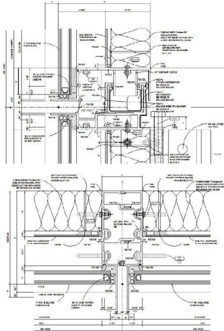
Figure 4. Typical horizontal and vertical stack joints.
