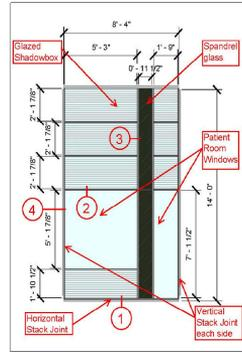
Figure 3. Typical unitized curtain wall panel.
