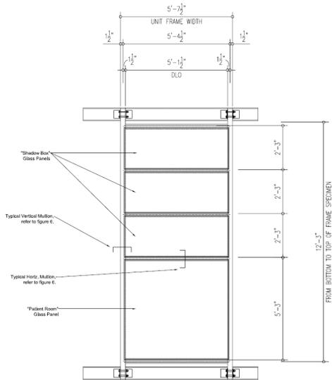
Figure 5. Mockup designed for preliminary testing.
