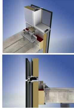
Figure 1. Rendering of stack joints and anchor system.
