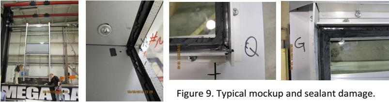
Figure 9. Typical mockup and sealant damage.
