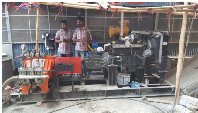
(b) High Pressure Jet Grout Pump System
