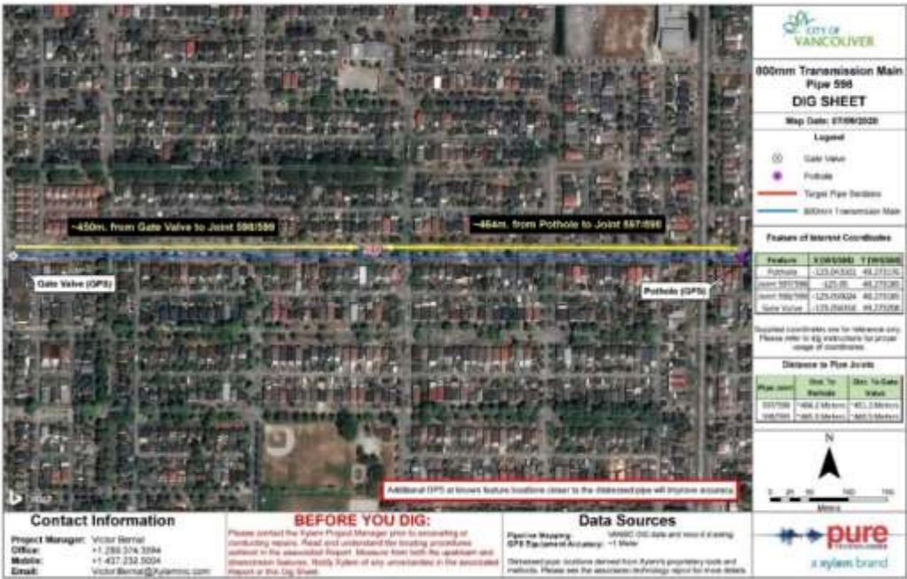
Figure 8. Example of dig sheet generated to pinpoint pipe sections with wall loss
