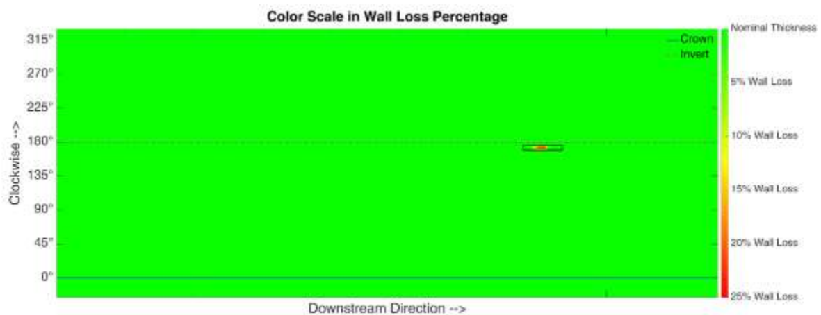
Figure 9. Heat map generated with the ultrasonic condition assessment tool data
