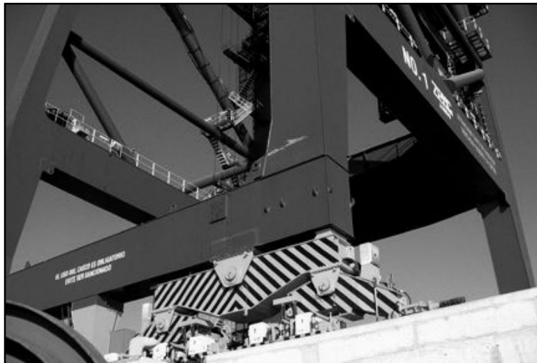
Figure 4.59 South Pier Container Crane with Impact Damage from Moored Vessel Impact (Vessel – Structure Interaction)
