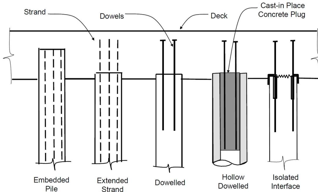
**Figure 3. Prestressed concrete pile connections.**
