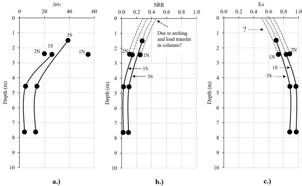
Figure 7: a.) Inferred changes in vertical effective stress in clay from subsurface deformations; b.) inferred SRR; c.) inferred stress efficacy
