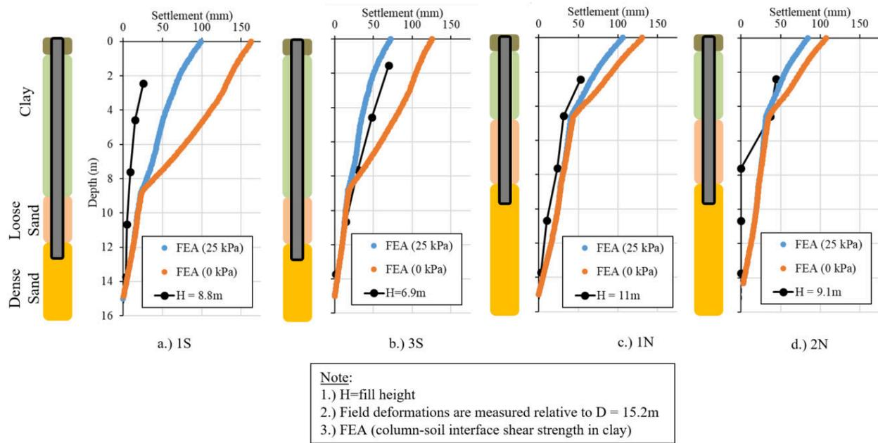
Figure 10: Computed and observed subsurface deformations with varying interface shear strength in clay
