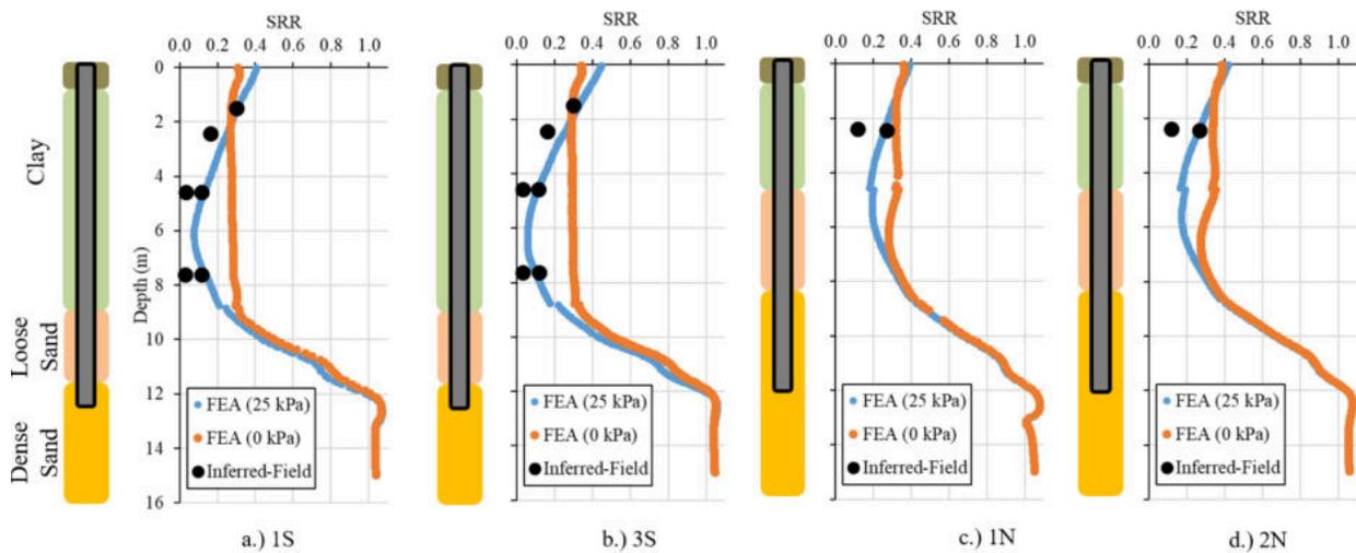
Figure 11: Computed and inferred SRR with varying interface shear strength in clay
