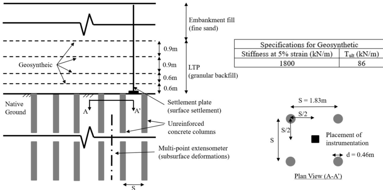
**Figure 3: Arrangement of columns, LTP/geosynthetic, and instrumentation**
