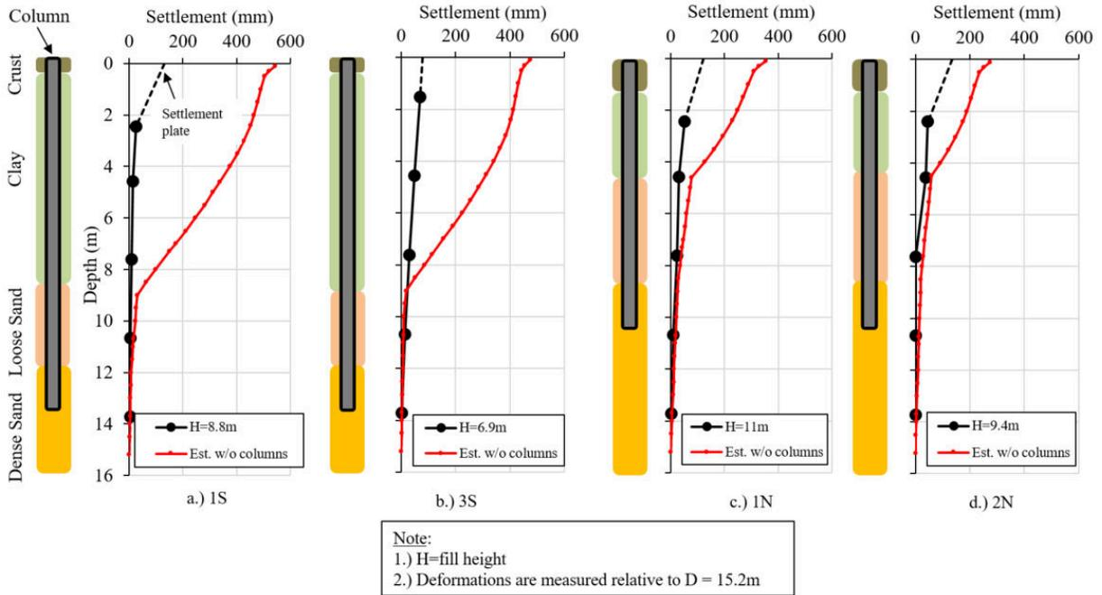
**Figure 5: Comparison of observed subsurface deformations with GRCS and estimated deformations *without* implementation of GRCS**
