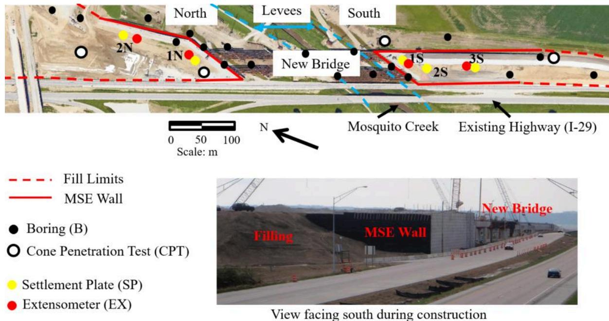
**Figure 2: Site details and fill/column limits for bridge construction**
