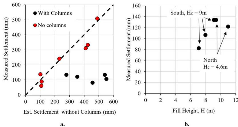
**Figure 6: a.) Settlement with and without columns; b.) Settlement vs. fill height**
