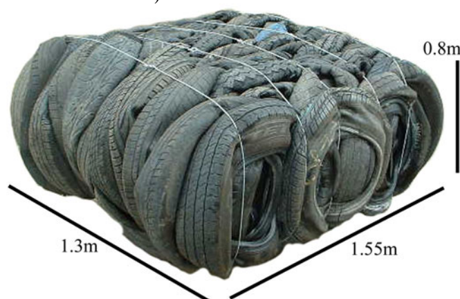
FIG. 1. A typical tyre bale with dimensions.
