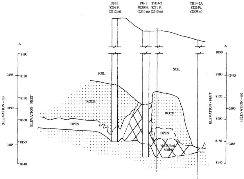
Figure 3. Geologic profile of the cavity complex
