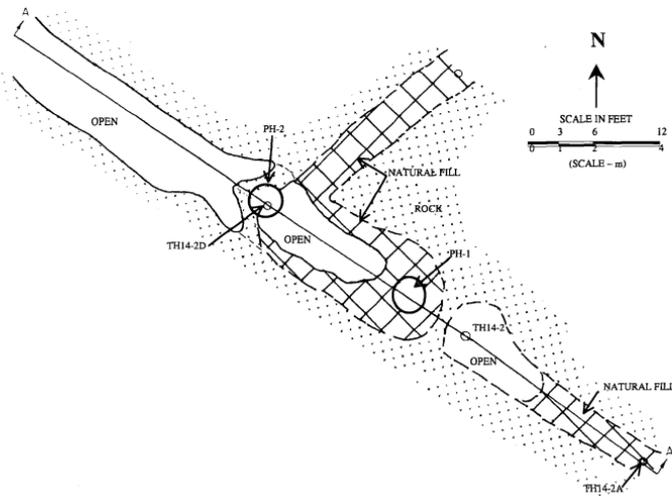
Figure 4. Geologic map of the cavity complex
