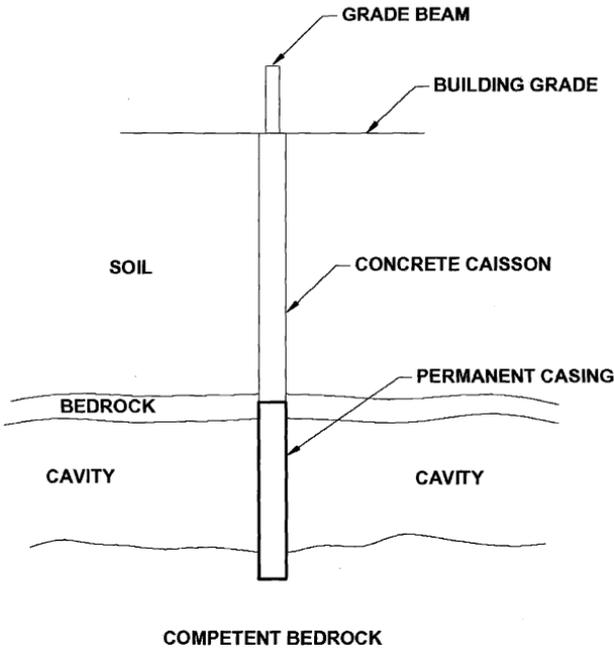
Figure 5. Example of permanently cased hole
