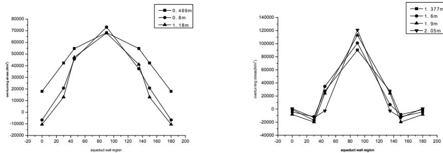
**FIG. 3. Variation curve of overturning stress extreme value for aqueduct wall region**
