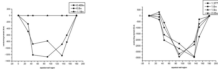
**FIG. 5. Variation curve of overturning moment extreme value for aqueduct wall region**
