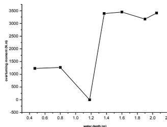
**FIG. 6. Variation curve of overturning moment extreme value along with water depth**
