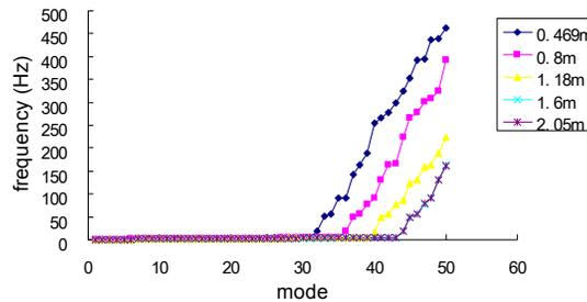
**FIG. 2. Frequency distribution curve of U-shaped aqueduct –fluid coupling system**
