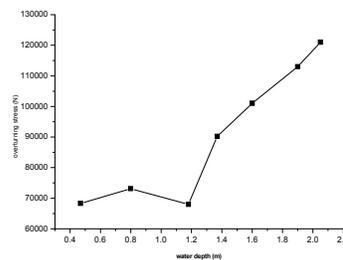
**FIG. 4. Variation curve of overturning stress extreme value along with water depth**
