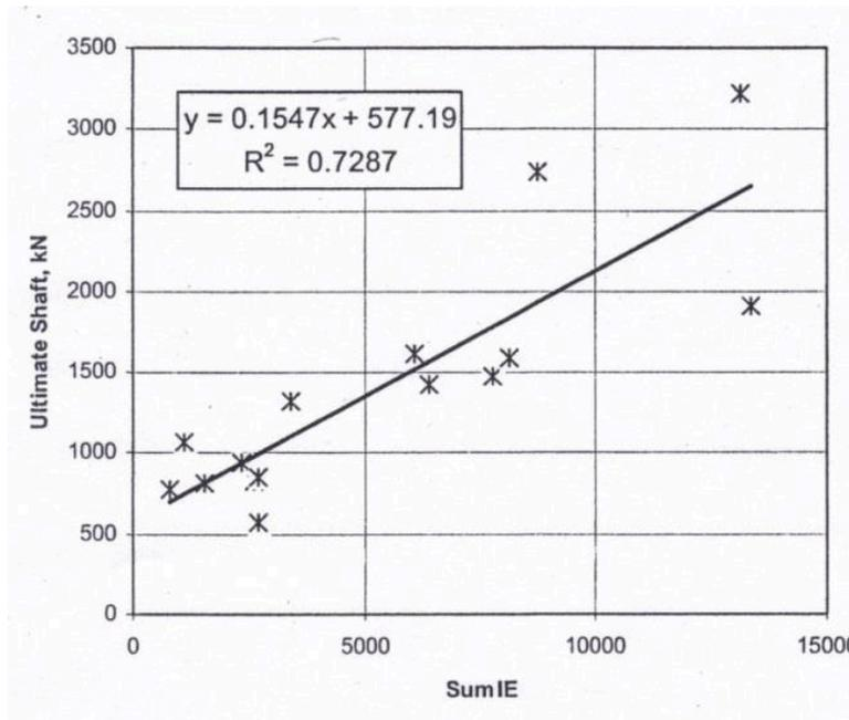
**Figure 2. Relationship Between Installation Energy and Side Resistance of ACIPD Piles. (from Nesmith 2003)**
