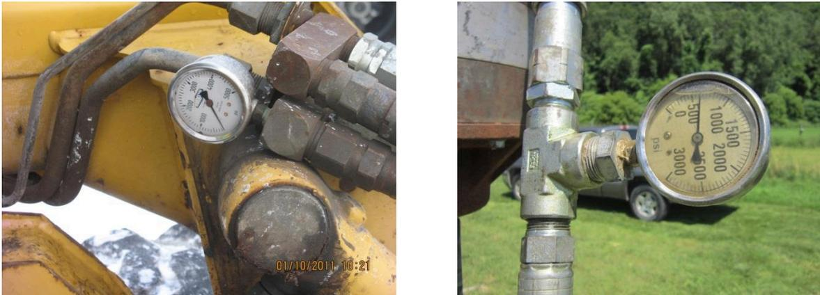
**Figure 3. Examples of Indirect Torque Measurement Using Hydraulic Pressure.**
