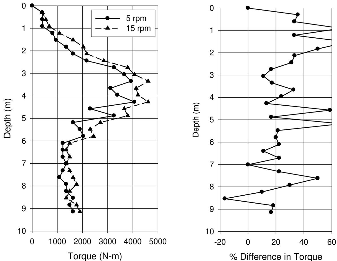
**Figure 5. Influence of Rotation Rate on Measured Torque.**
