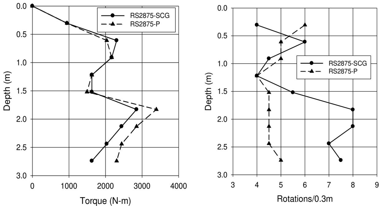
Figure 6. Installation Torque and Advance for two Round Shaft Helical Anchors.
