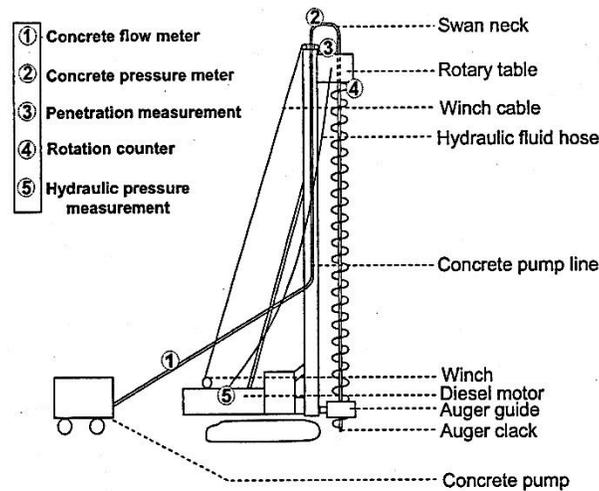
**Figure 1. Typical Instrumentation for Monitoring Construction of CFA, ACIP and ACIPD Piles.**
