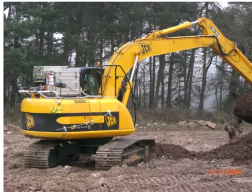
Figure 1: PEMS mounted on a nonroad equipment (Google 2017a)
