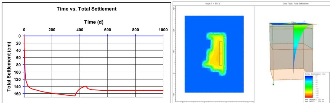
**FIG. 7. Settlements evolution with a PVD improvement before and after the building construction.**
