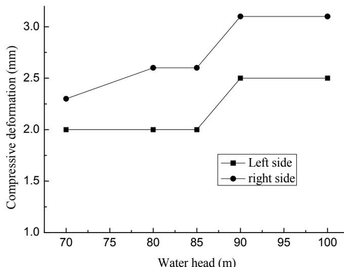
**FIG. 5. Correlation of the water head and the preset compressive deformation of the rotation hinge seal**
