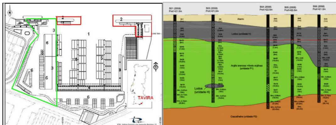
**FIG. 4. Layout of the Tavira fishing harbour, with a geotechnical profile along the breakwaters; in grey, soft to very soft clays, in green clays, clayey sands and sandy clays, and brown are gravels, with  $N_{SPT}$  greater than 60.**
