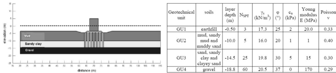
FIG. 5. Geotechnical profile and solution in stone columns for the breakwaters foundation reinforcement and the geotechnical parameters used in FEM.
