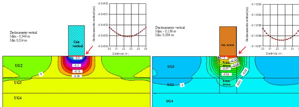
FIG. 6. Settlements by FEM analysis at the base of the quay, without and with soil reinforcement, respectively maximum of 54 cm and 13 cm.
