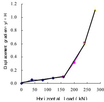
**Fig. 3 Horizontal force and force displacement gradient of #b<sub>2</sub>' pile**
