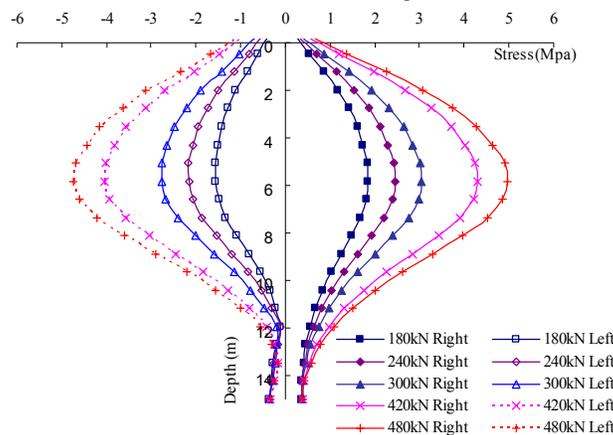
**Fig. 6 Stress distribution curve of pile body under load of every level**
