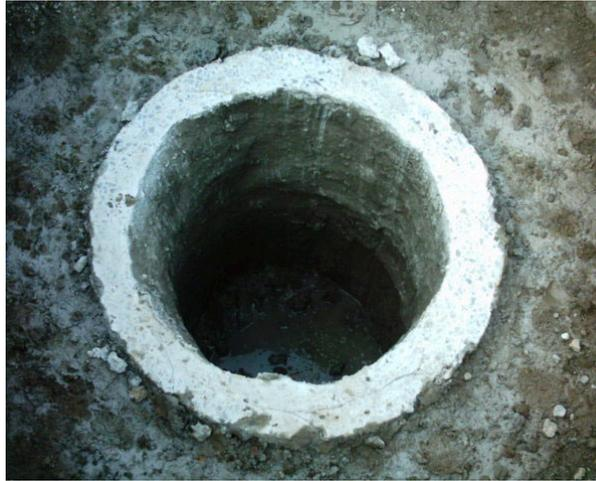
**FIG.3** Photo of excavated test pile
