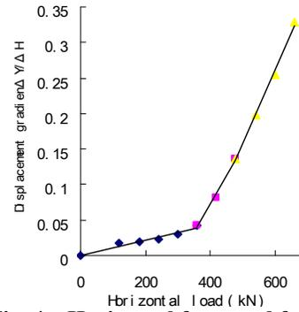
**Fig. 4 Horizontal force and force displacement gradient of #a<sub>1</sub>' pile**
