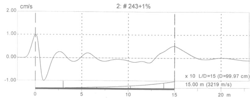
**FIG.4** Wave shape of the small strain test
