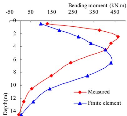
**Fig. 7 Comparison curve of calculated bending moments and measured ones, H=180kN**
