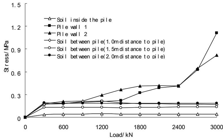
FIG.6 Stress in composition bearing test
