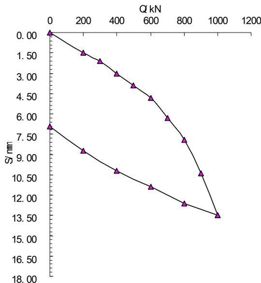
**FIG.5 Q-S curves of test pile**
