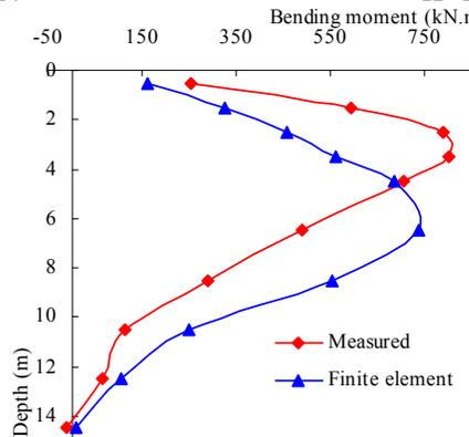
**Fig. 9 Comparison curve of calculated bending moments and measured ones, H=300kN**
