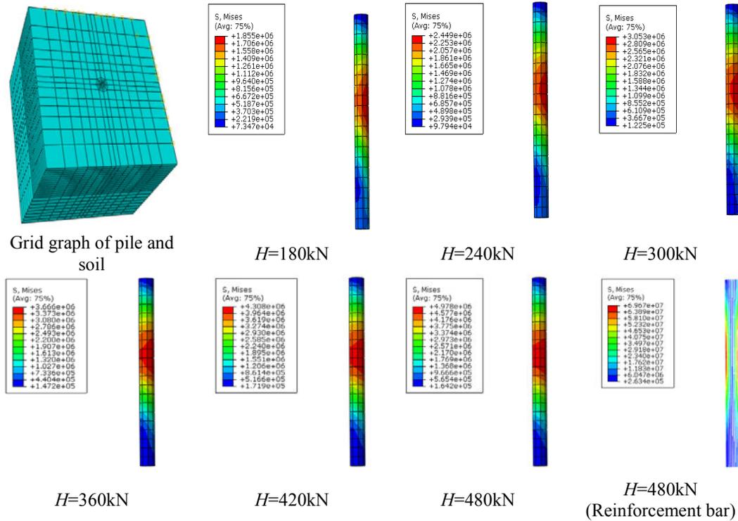
**Fig. 5 Grid graph and stress distribution nephogram of pile body and reinforcement bar under load of every level**
