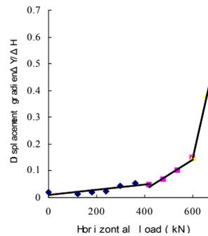
**Fig. 2 Horizontal force and force displacement gradient of #a<sub>1</sub> pile**
