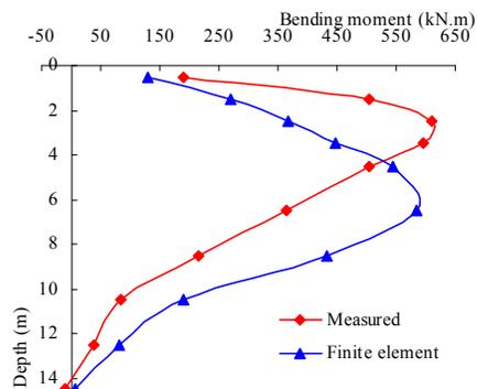
**Fig. 8 Comparison curve of calculated bending moments and measured ones, H=240kN**
