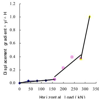
**Fig. 1 Horizontal force and force displacement gradient of #b<sub>2</sub> pile**
