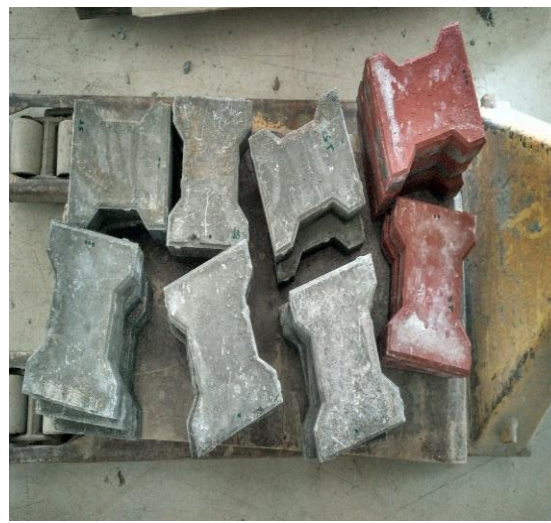
Figure 8: Dried paver blocks
