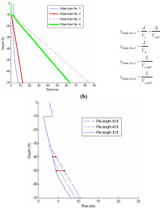
**Fig. 5** (a) the predicted first arrival of different wave trains using the propagation paths shown in Figure 4, (b) the sensitivity of the first arrival on the pile length.
