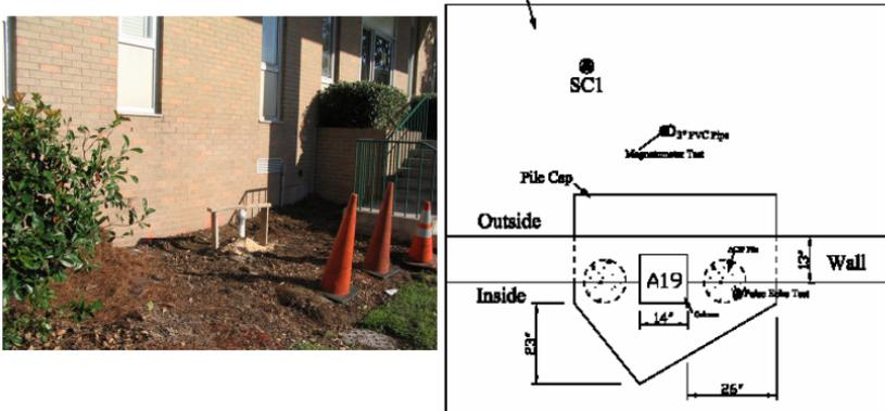
**Fig. 2** (a) view of outside building (b) plane view of Column A19 and locations of drilled shaft
