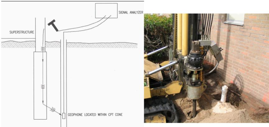
**Fig. 3** a) Schematic of Parallel Seismic Testing; b) Parallel Seismic Test Using SCPTu
