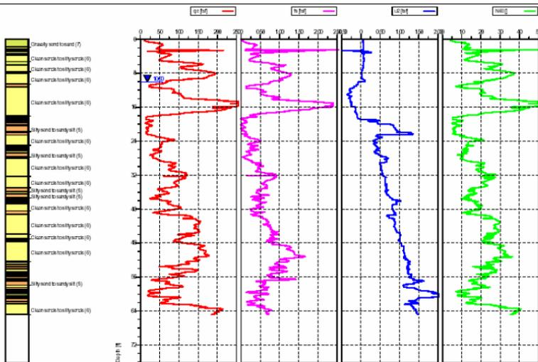
Fig. 1 Example Results of CPTu Test
