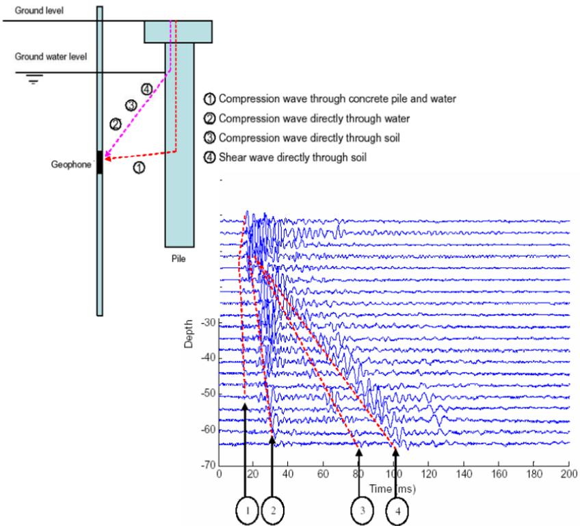
**Fig. 4** Recorded signals at A3 with wave trains identified (the possible wave train propagation paths and modes are shown in the schematic drawings)
