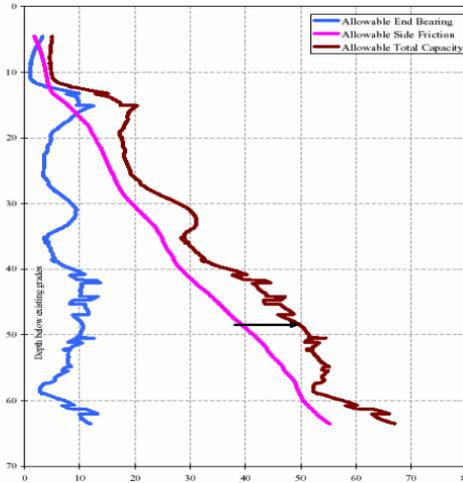
**Fig. 6** Pile Net Bearing Capacity With Depth using French Method
