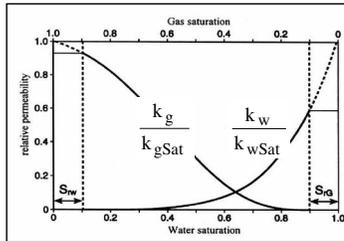
**FIG 5. Schematic relative permeability with respect to fluid saturation (Warrick, 2002)**
