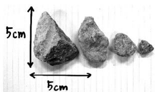
FIG. 1. Waste concrete aggregate used in the experiment.
