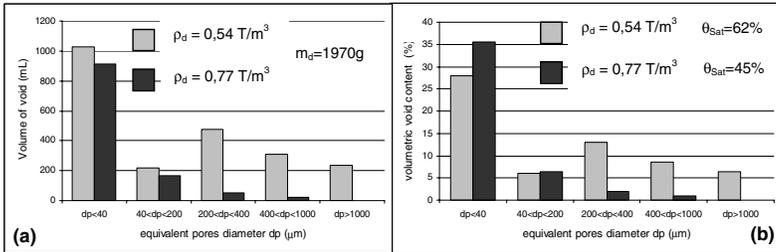
**FIG 8. (a) Volume of void versus equivalent pores diameter of the drilled domestic waste at two dry densities, for a given mass of waste, (b) Volumetric void content versus equivalent pores diameter of the drilled domestic waste at two dry densities (corresponding to a given unit overall volume of waste)**
