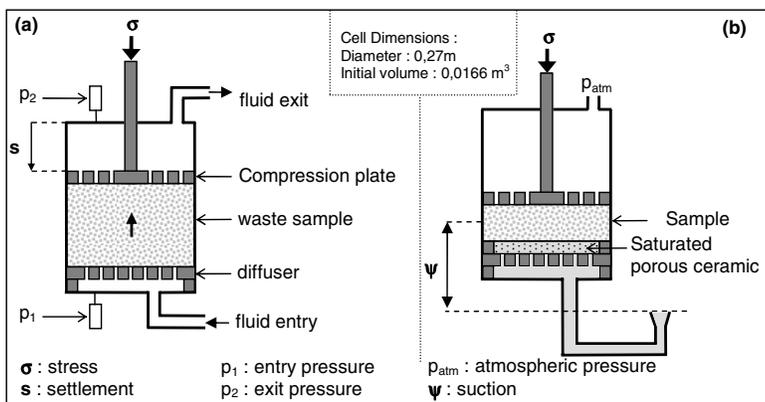
FIG 2. (a) Schematic section of the compression cell of the oedopermeameter equipped for the gas permeability test , (b) Schematic section of the modified oedopermeameter compression cell equipped for the suction test
