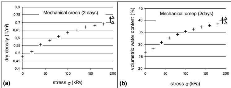
**FIG 3. (a) Evolution of the dry density versus the compression vertical stress, (b) Evolution of the volumetric water content versus the compression vertical stress**
