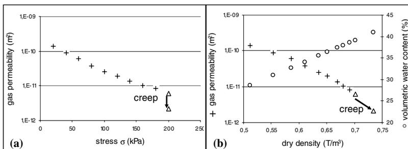
**FIG 4. (a) Evolution of the gas permeability versus the compression vertical stress, (b) Evolution of the gas permeability versus the dry density**
