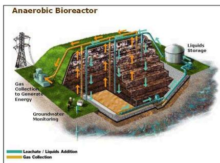
FIG 1. General schema of a bioreactor (Ademe source)
