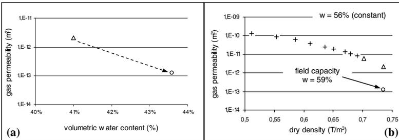
**FIG 6. (a) Evolution of the gas permeability versus the volumetric water content after a saturation-desaturation cycle (field capacity state), (b) Evolution of the gas permeability during the phase of compression and after a saturation-desaturation cycle (field capacity state)**
