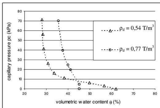
**FIG 7. Water retention curve of the drilled domestic waste at two dry densities**
