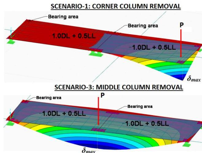
**Figure 3: Element removal scenarios: corner column (top) and middle column (bottom)**
