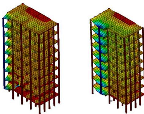
**Figure 4: Deformed shape: Column-5 removal (left) Column-6 removal (right)**
