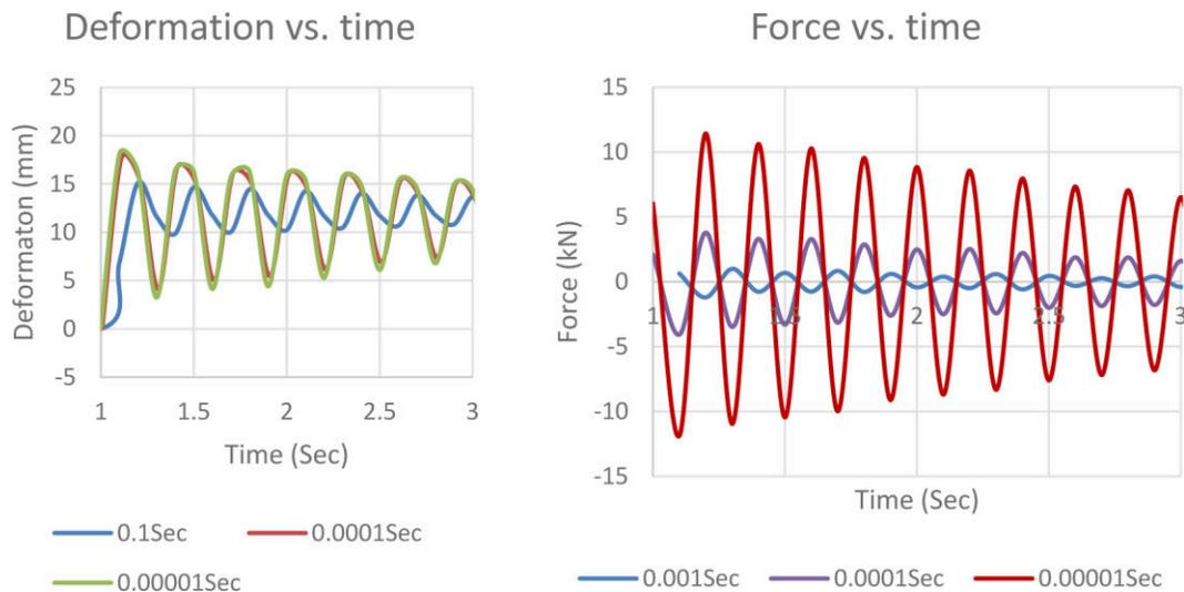
**Figure 5: Column-5 removal: Deformation vs. time (left) and Force vs. time (right)**
