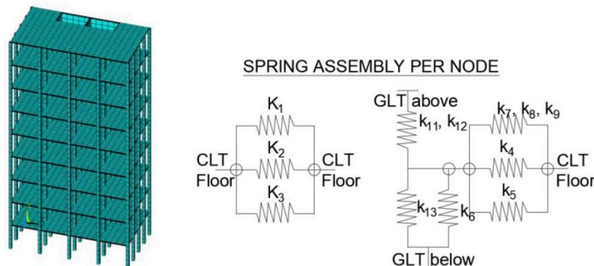
**Figure 2: FE model of the 12-storey building (left), floor-to-floor connection (Centre), and column-to-column and floor to column connection (right)**
