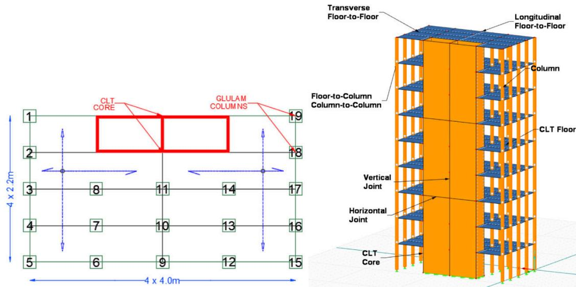
**Figure 1: Building floor plan (left) and isometric view (right)**
