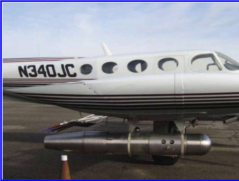
Fig. 5-2. Example of an acetone-silver iodide generator mounted on a wing tip Source: Courtesy of North American Weather Consultants, Inc.
