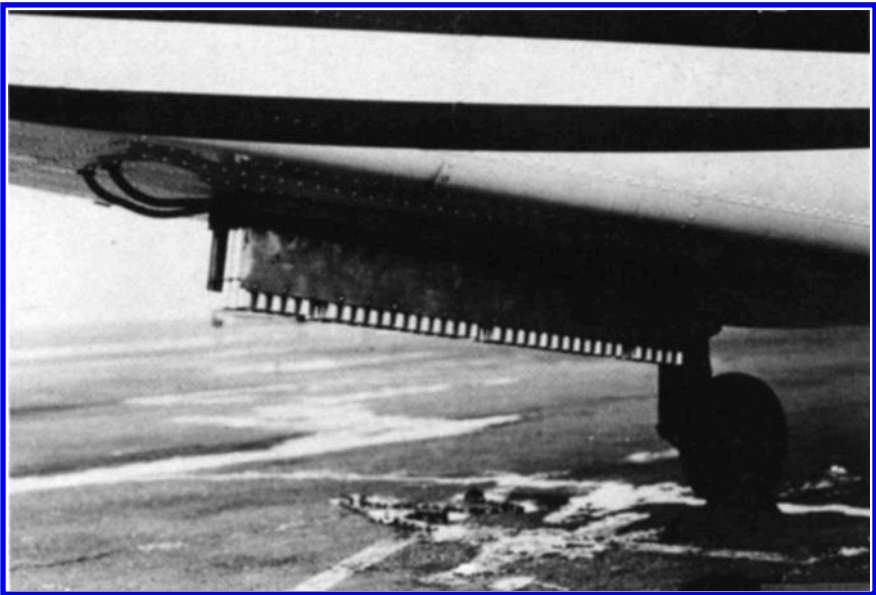
Fig. 5-4. Example of an ejectable silver iodide pyrotechnic rack Source: ASCE (2004); © ASCE.
