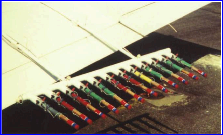
Fig. 5-3. Example of a wing-mount silver iodide pyrotechnic rack Source: Courtesy of Weather Modification, Inc.
