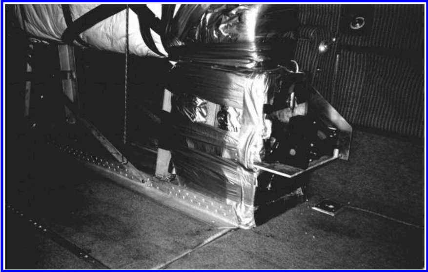
Fig. 5-5. Example of a dry ice dispenser mounted in an aircraft Source: ASCE (2004); © ASCE.
