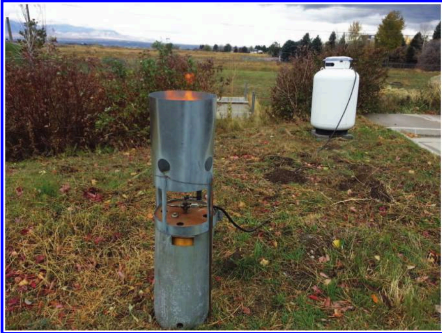
Fig. 5-6. Example of a manually operated, ground-based silver iodide generator Source: Courtesy of North American Weather Consultants, Inc.
