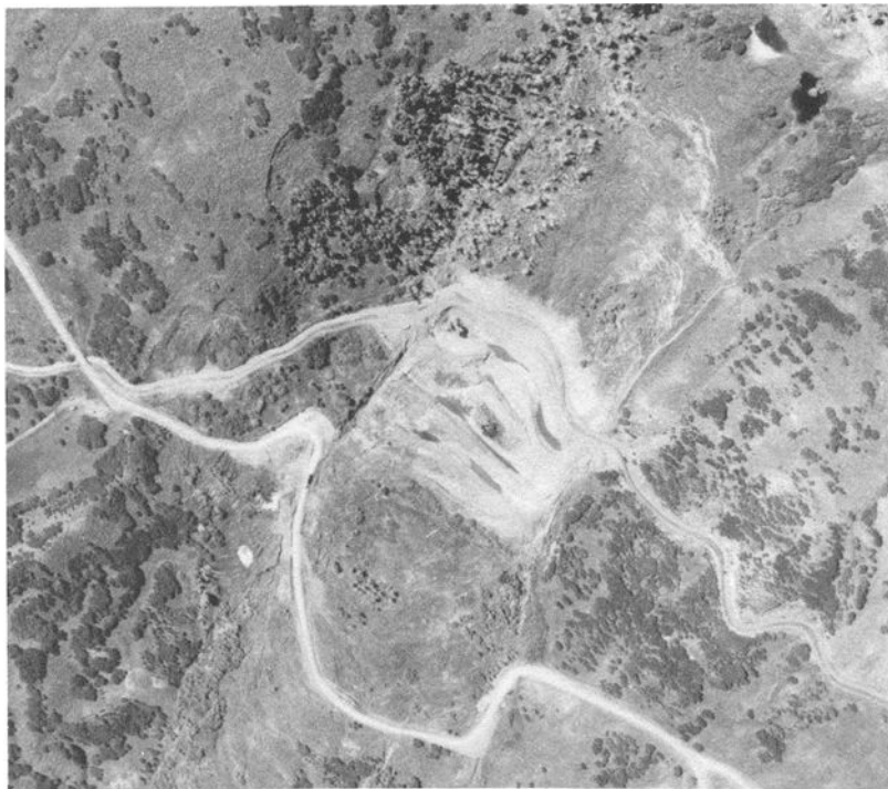
Figure 3. Portion of reactivated earth slide - earth flow showing multiple abandoned canal sections, cracking, and sag ponds. Note 18-wheel truck on road for scale. Movement is from top right to bottom left of photograph.
