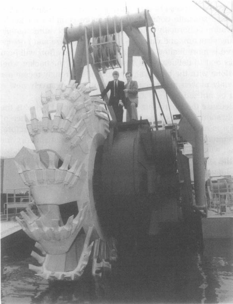
Fig. 13-11. Rennison Goldfield's 1,340 HP bucketwheel. Courtesy: IHC.
