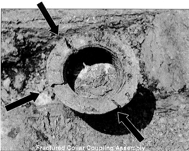
Photograph 3 – Delineating Through-Wall Cracking
