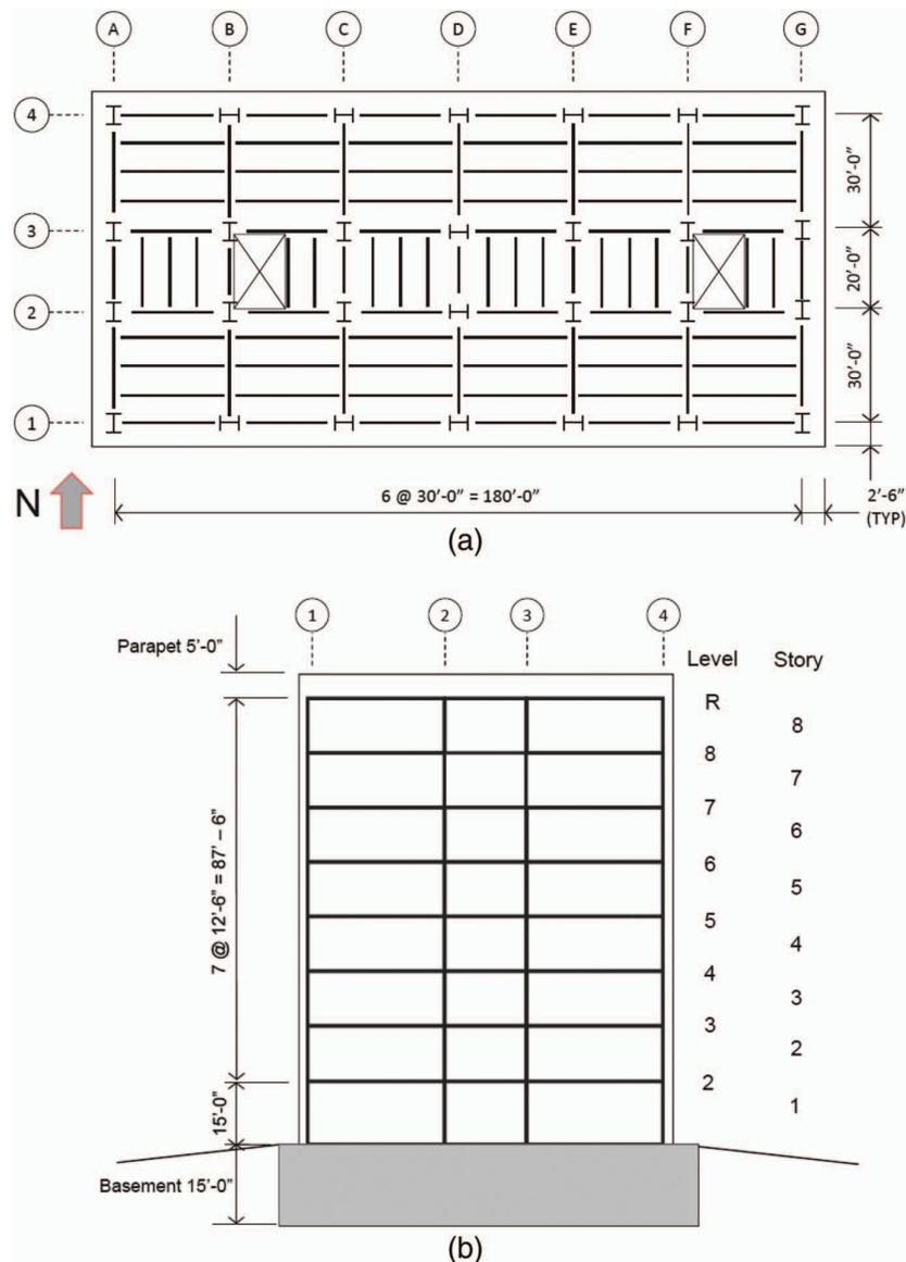
**Figure G21-1.** Plan and elevation of the 8-story building.
