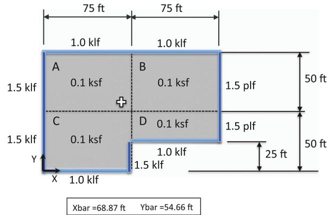
**Figure G20-6. Floor plate dimensions, weights, and subplate designations.**
