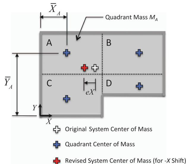
**Figure G20-5. Diaphragm mass divided into four quadrants.**
