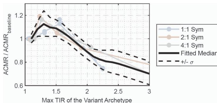
**Figure G20-8. Results from the FEMA P-2012 report regarding use of mass offset versus static torsion.**
