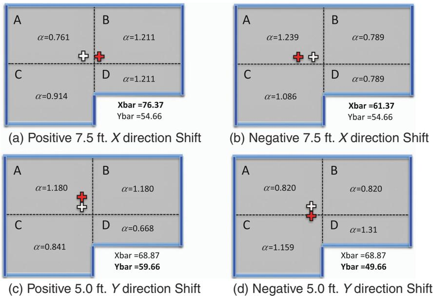
**Figure G20-7. Mass adjustment factors and revised centers of mass.**
