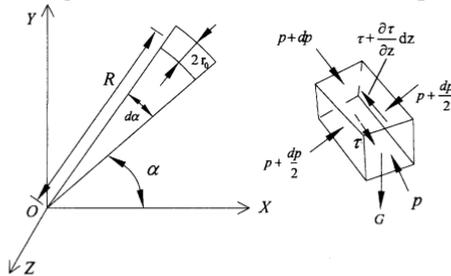
Fig.1 Forces on fluid microelement from  $\theta=45^\circ$  to the upward and corresponding coordinate system
