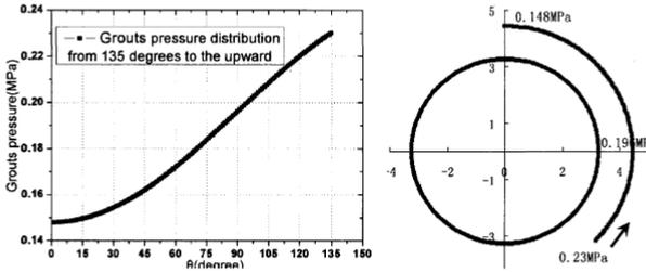
**Fig.4 Pressure distribution from  $\theta=135^\circ$  to the upward**
