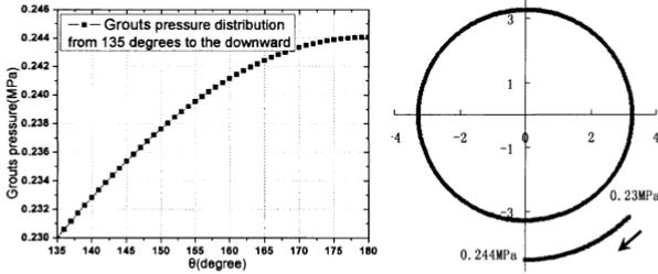
**Fig.5 Pressure distribution from  $\theta=135^\circ$  to the downward**
