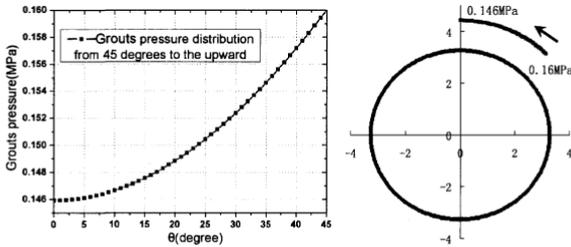
**Fig.2 Pressure distribution from  $\theta=45^\circ$  to the upward**
