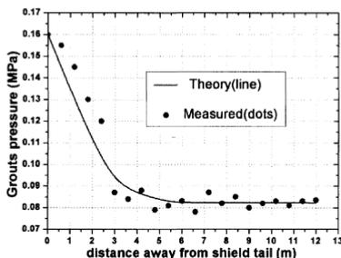
Fig.7 Final distributions of grouts pressure in longitudinal section at  $\theta = 45^\circ$
