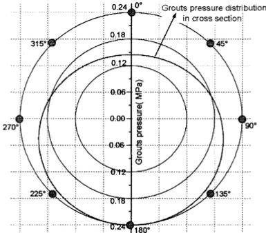
**Fig.6 Final distributions of grouts pressure in cross section.**
