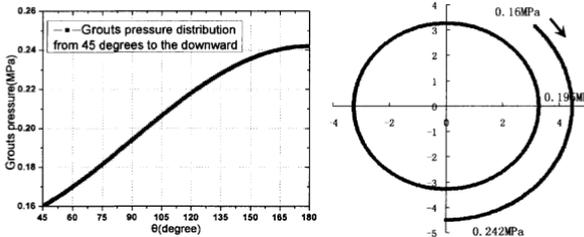
**Fig.3 Pressure distribution from  $\theta=45^\circ$  to the downward**
