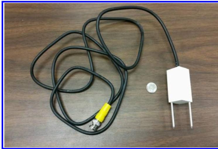
**FIG. 2. Photo of the moisture-suction TDR probe.**
