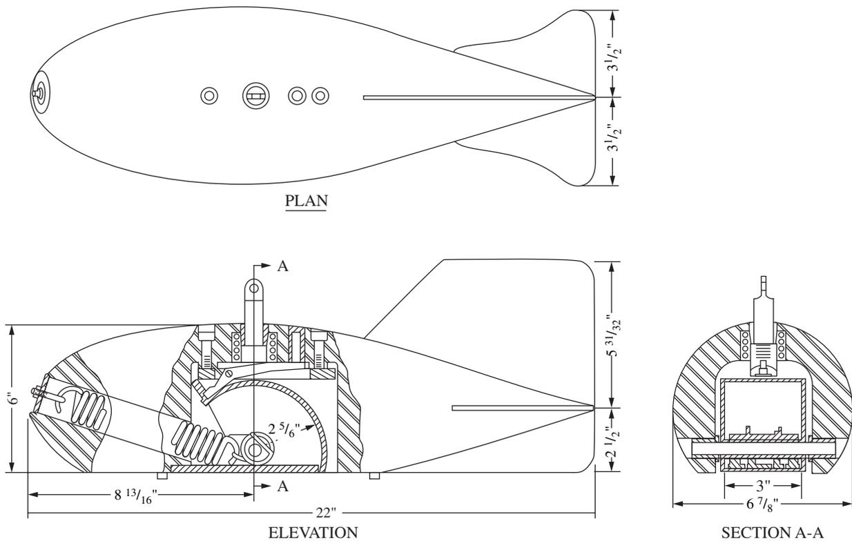
Figure 3.19 US BM-54 bed material sampler (Interagency Committee, 1963).
