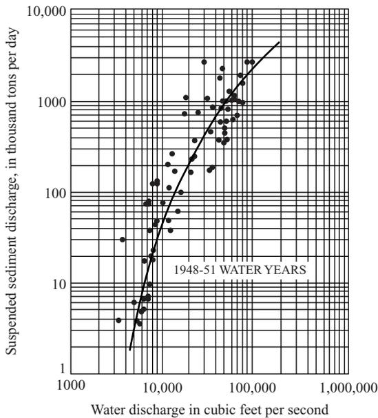
**Figure 3.28** Suspended-sediment transport curve, Colorado River near Grand Canyon, Arizona.
