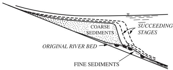
**Figure 3.30** Profile of typical reservoir delta.
