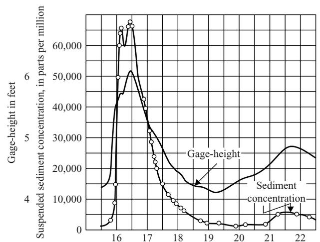
**Figure 3.27** Graphs of suspended-sediment concentration and gage height, Bighorn River near Manderson, Wyo., April 16–22, 1952.
