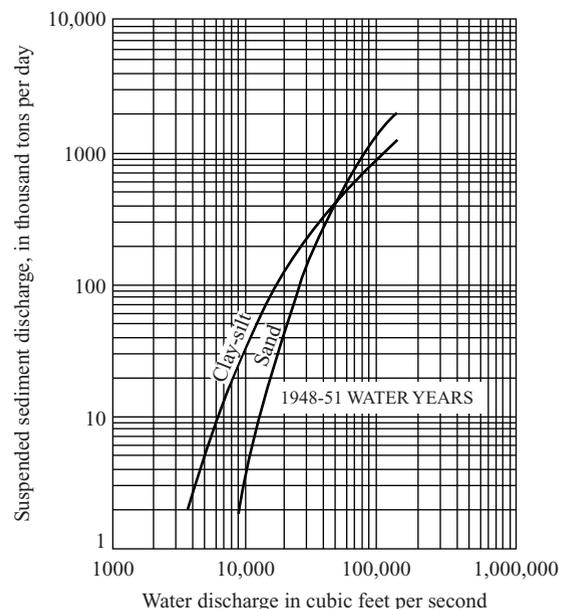
**Figure 3.29** Suspended clay-silt and sand transport curves, Colorado River near Grand Canyon, Arizona.
