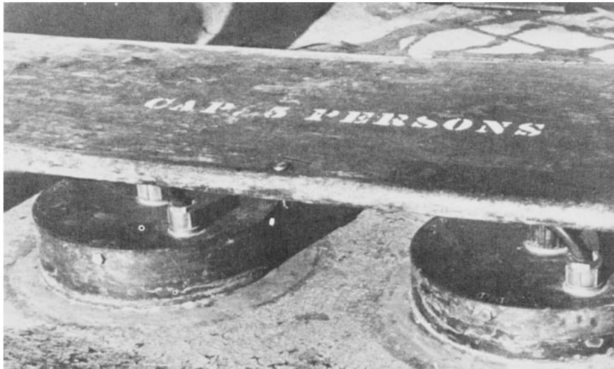
**Figure 3.31** Transmitting and receiving transducers mounted in boat hull (Photograph by United States Bureau of Reclamation).
