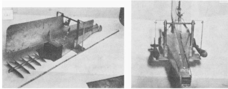
**Figure 3.26** Experimental bed load sampler: (A) View of sampler with baffles removed; (B) View of sampler with sounding weights attached (Photographs by United States Army Engineer District, Little Rock, Ark.).
