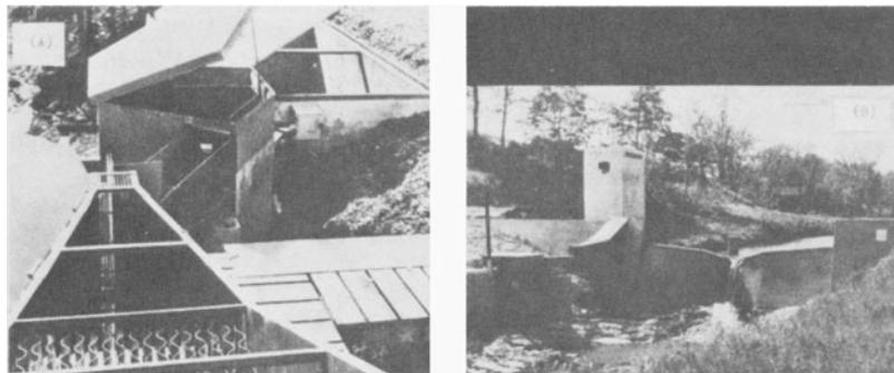
**Figure 3.25** Streamflow and sediment measuring station, White Hollow Creek near Maynardville, Tenn.: (A) Flow splitting device with water-sediment storage tank; (B) Looking upstream—weir in immediate foreground, flow splitting device at left (Photographs by Tennessee Valley Authority).
