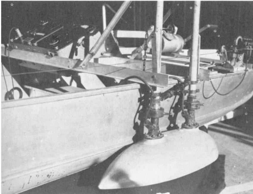
**Figure 3.32** Transducer attached to side of boat (Photograph by United States Bureau of Reclamation).
