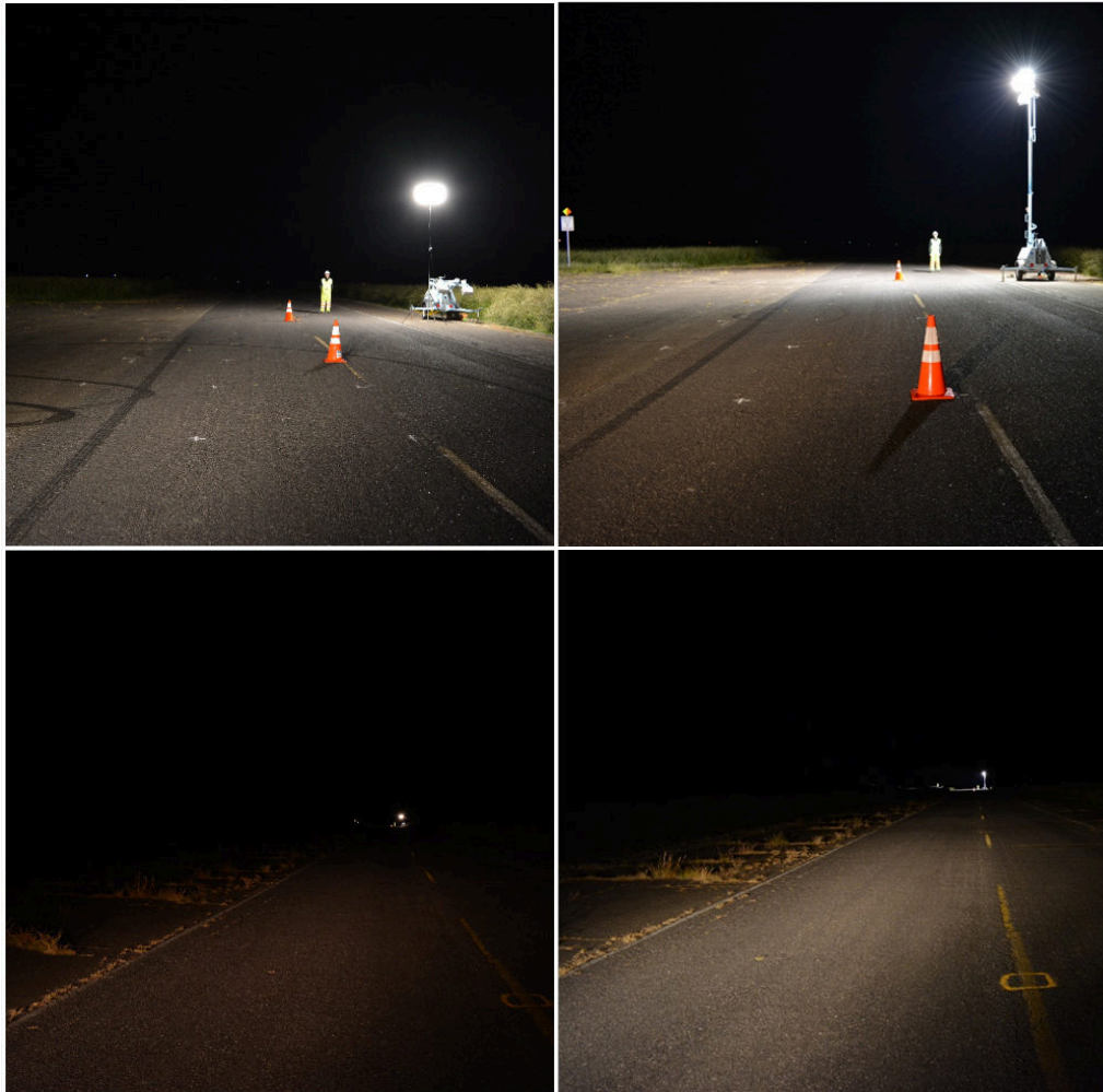
Figure 1. Worker at Different Distances from Light Source (a) top left, 100 feet Balloon Light; (b) top right, 100 feet Light Tower; (c) bottom left, 1000 feet Balloon Light; (d) bottom right, 1,000 feet Light Tower
