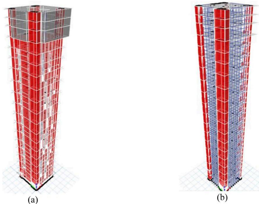
**Fig. 1. ETABS models of the tower. (a) Shear wall system (b) Tubular system.**
