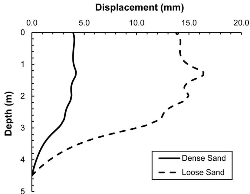
**Figure. 6 Comparison of displacement for the helical pile with three helices in dense and loose sand conditions**
