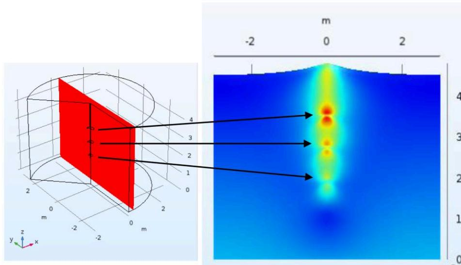
**Figure. 4** Stress distribution in the specific soil plane beside the helical pile.
