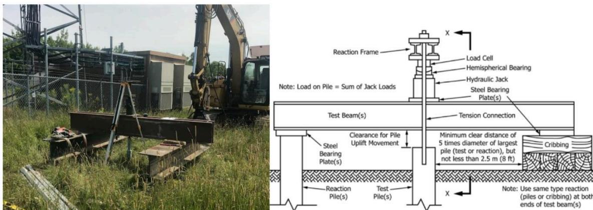
**Figure. 1 Tensile load test setup at the site and typical setup supported on test beams (ASTM 3689)**
