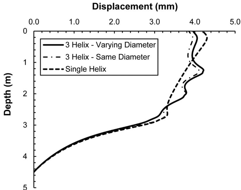
**Figure. 5 Displacement versus depth for three piles with different helix configurations – three helices of different diameters (0.20-0.25-0.30 m), single helix (0.20 m) and three helices of the same size (0.30 m)**
