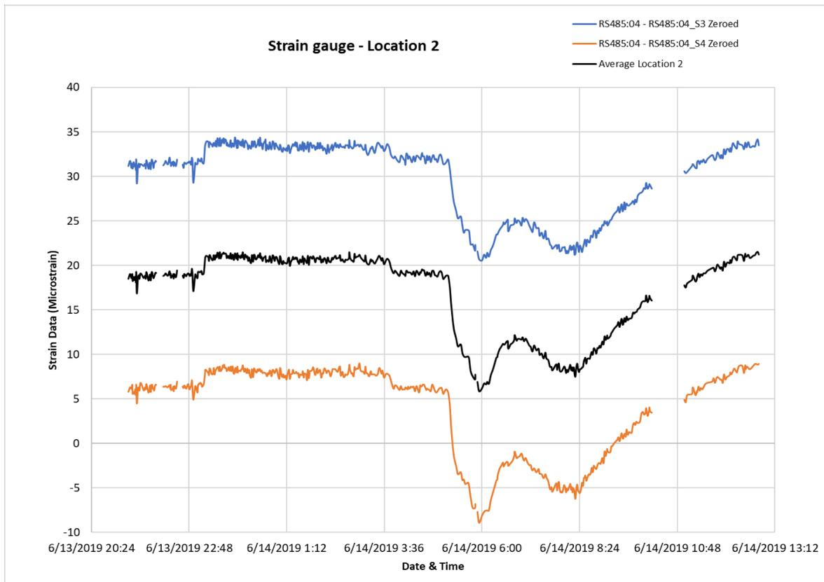
**Figure 11: Life cycle monitoring data collected for 24-hour period at Location 2**
