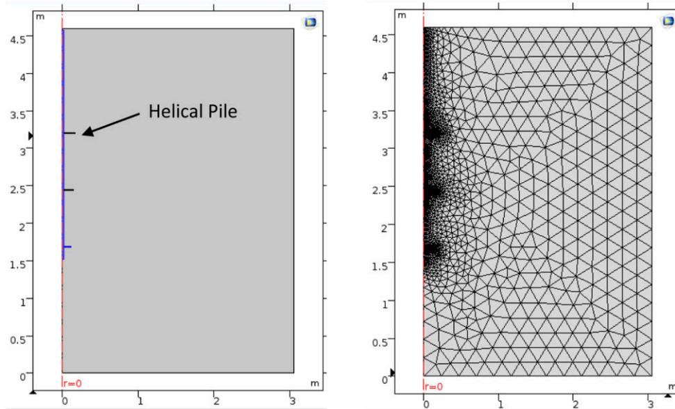
**Figure. 2 Modeling geometry and mesh**
