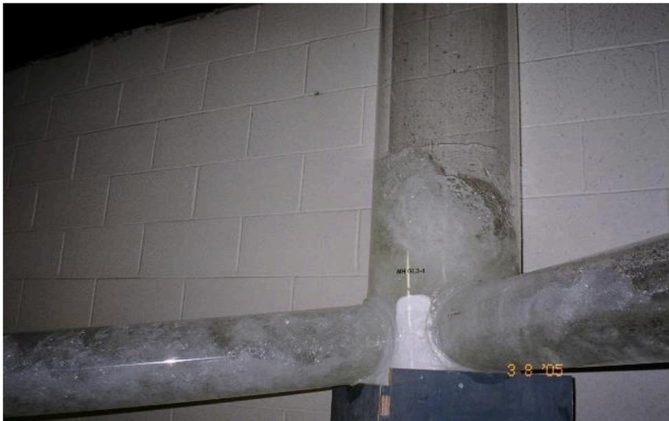
**Figure 5. Simulation of air transferred downstream due to a sharp alignment change through a maintenance hole.**
