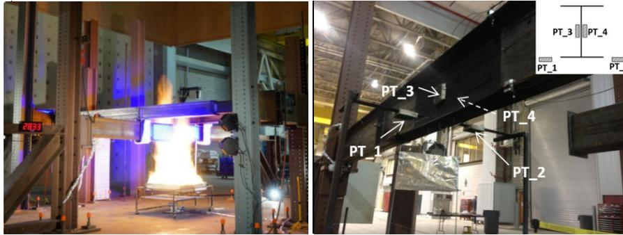
Figure 2 Test setup (left) and installation of plate thermometers (right)
