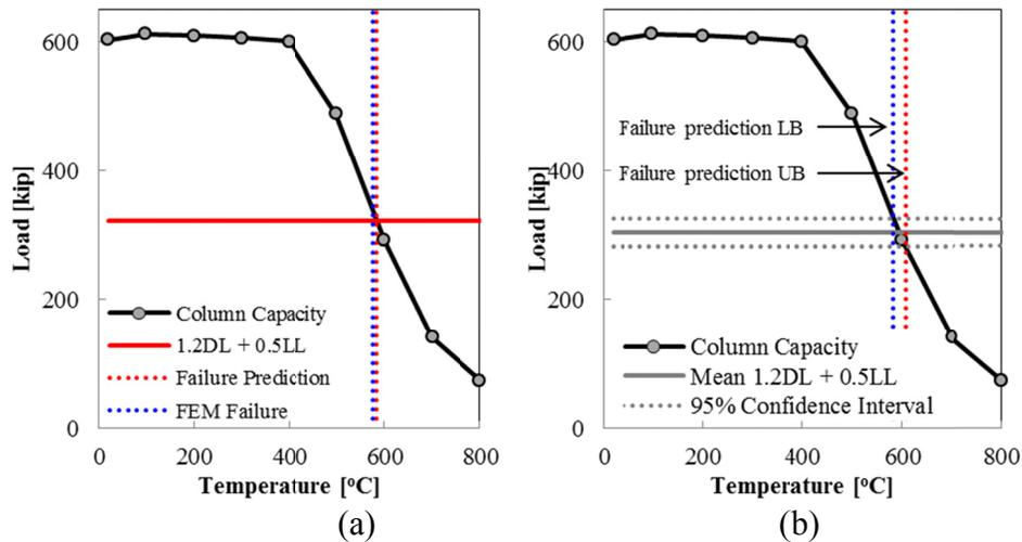
Figure 4 Column capacity varying with temperature for interior gravity column supporting the 6<sup>th</sup> floor (W12x58) (a) column capacity compared with column load and prediction temperature for failure, (b) column capacity compared with mean column load throughout building with 95% confidence interval for failure
