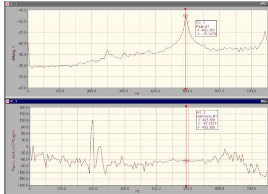
Figure 3: Frequency distribution of magnitude and phase of accelerations in loosening at 500 Hz
