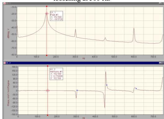
Figure 4: Frequency distribution of magnitude and phase of acceleration in tightening at 150 Hz
