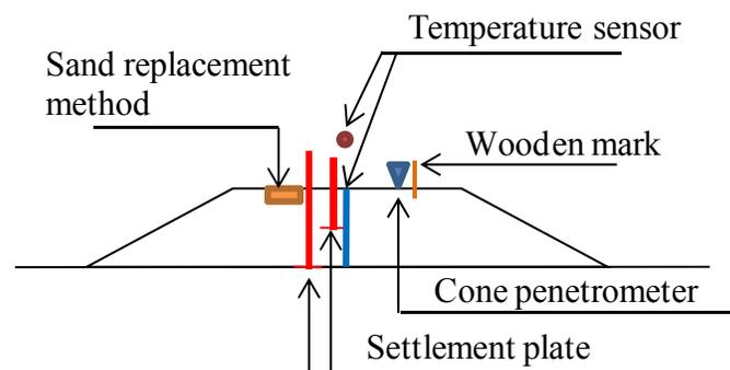
**Figure 3. The measurement position of the embankment.**
