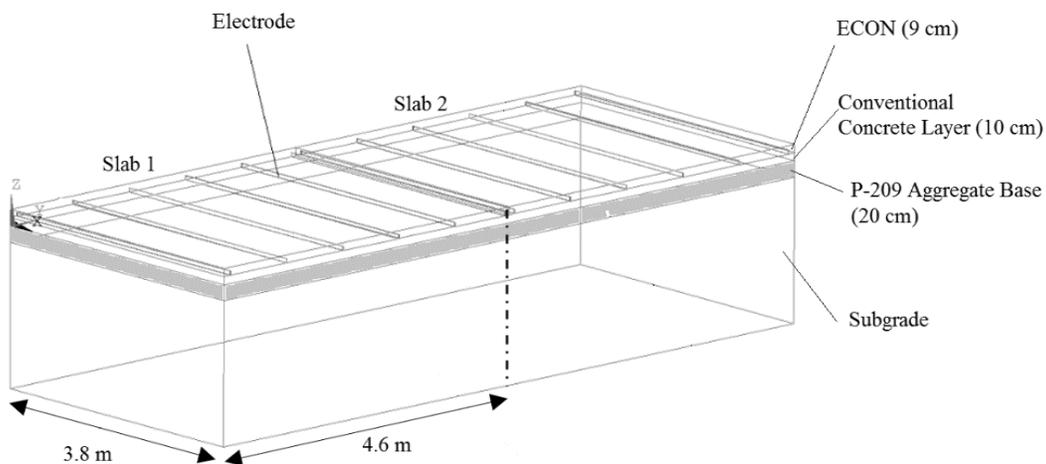
**Figure 1. Finite element model of the ECON slabs constructed at Des Moines International Airport**
