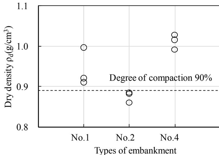
**Figure 4. Dry densities of the embankments immediately after construction.**
