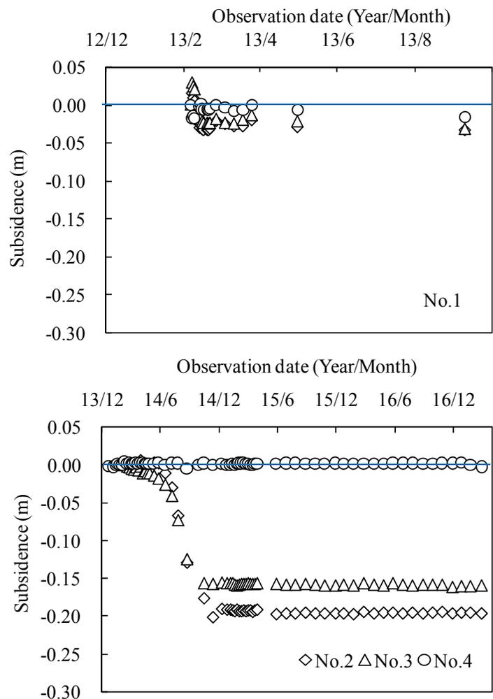
**Figure 6. Subsidence of embankment.**
