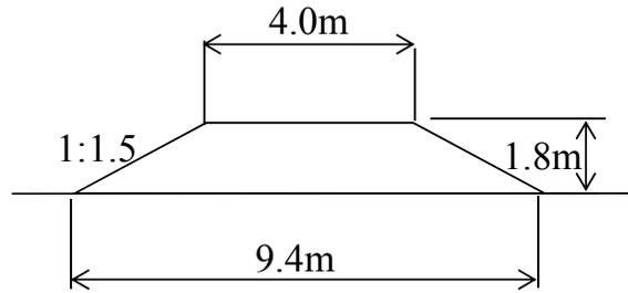
**Figure 2. Embankment shape.**
