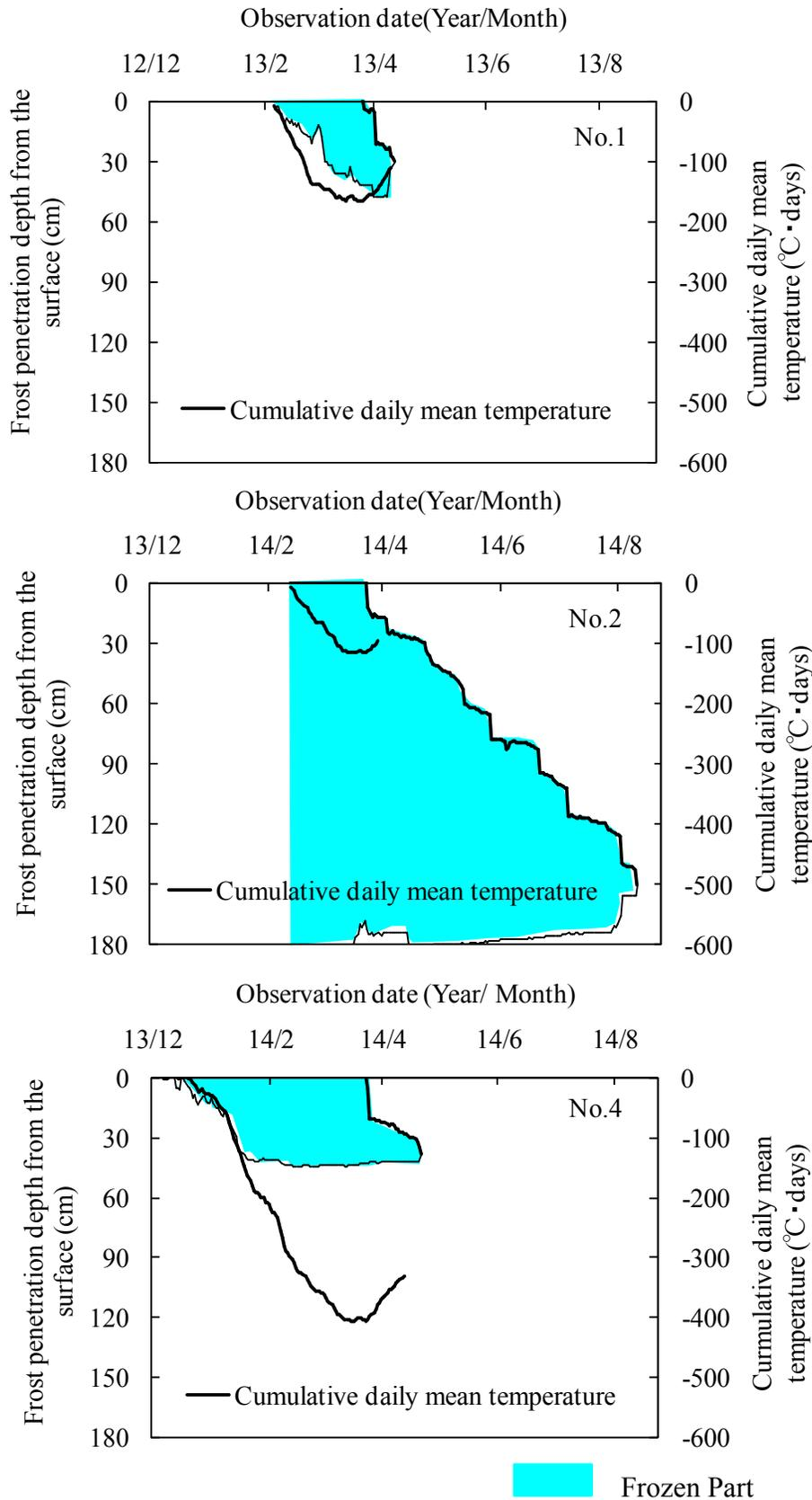
Figure 5. Frozen portion of embankment.
