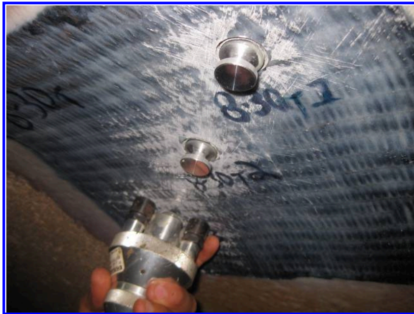
Figure 5. Pull Test per ASTM D4541
