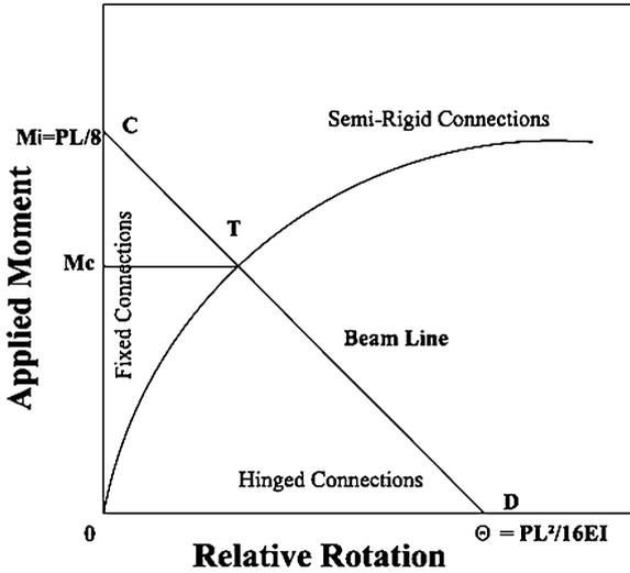
Figure 8-4. Beam-line method for semi-rigid connections analysis.
