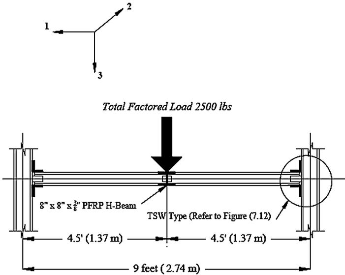
Figure 8-5. Details of the semi-rigid connected PFRP beam of Example 8-1.
