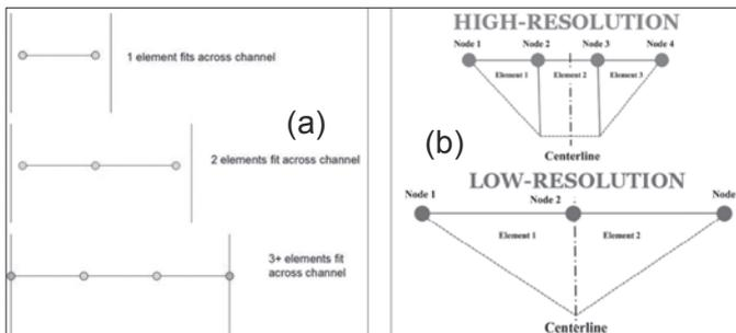
**Figure 2.** (a) Three different channel widths represented by fixed-size elements; and (b) *high-resolution* channel representation (actual channel width and trapezoidal cross-section) and *low-resolution* channel representation (artificially increased channel width and V-notch cross-section).
