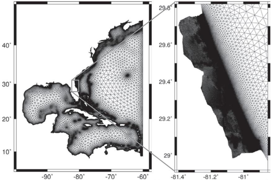
**Figure 4.** Large-scale finite element mesh with Intracoastal Waterway in north Florida at high resolution.
