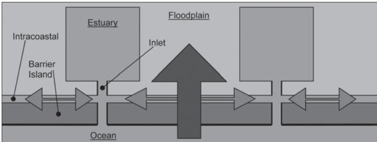
**Figure 1.** Local plan view of Intracoastal Waterway and other coastal features (labeled). Arrows indicate perpendicular surge overflow ( $\uparrow$ ) and along-channel surge conveyance ( $\leftrightarrow$ ).
