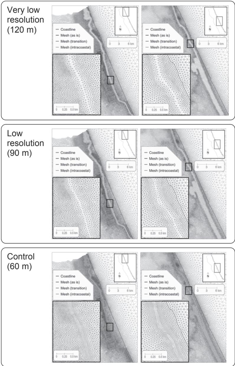
Figure 5. Five finite element meshes for the Intracoastal Waterway in north Florida.
