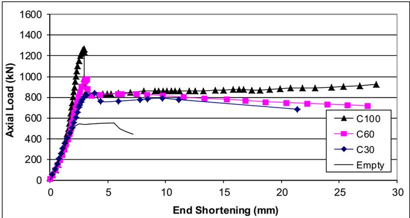
Figure 4: Axial load vs. end shortening curves for 150x75x4 EHS composite columns
