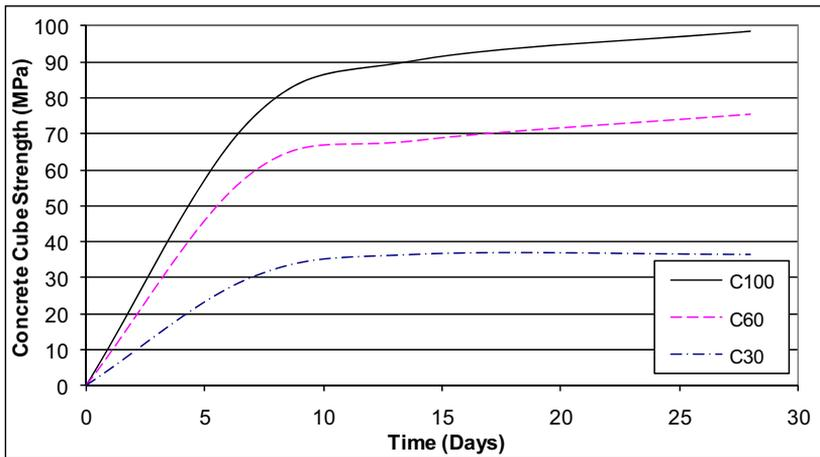
**Figure 2: Concrete development strength**
