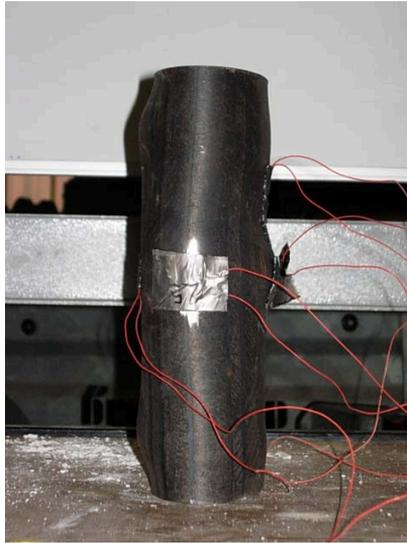
**Figure 3: Typical failure mode of the composite EHS**
