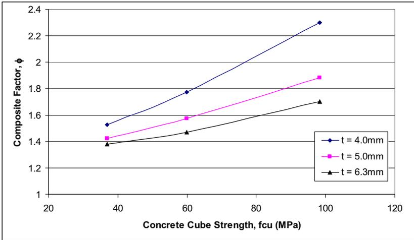
Figure 7: Composite factor vs. concrete cube strength curves
