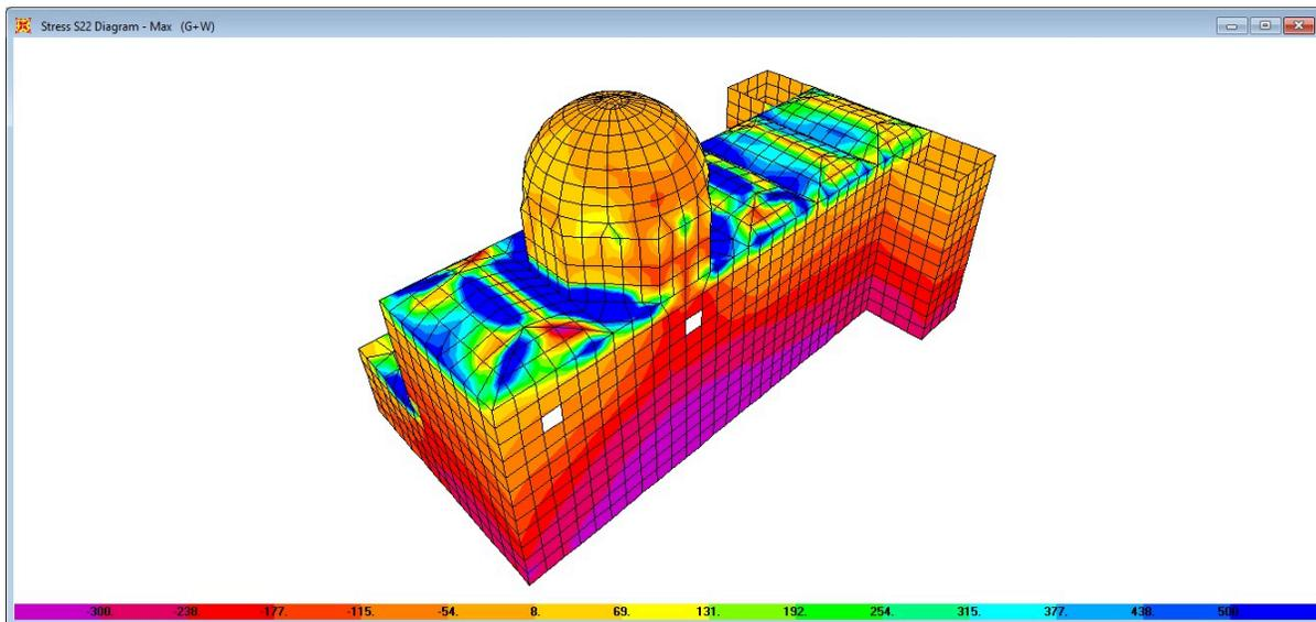
**Figure 8. Compression and tensile stress distribution due to gravity and wind analysis in the repaired structure.**
