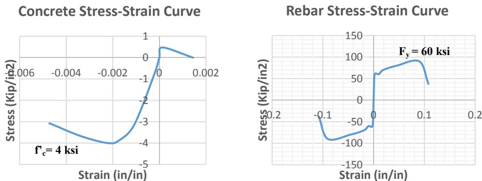
**Figure 4. Typical idealized stress-strain behavior.**
