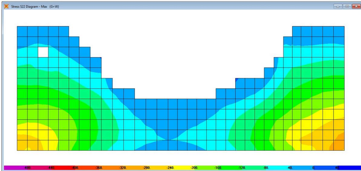
**Figure 9. Compressive stress distribution due to gravity and wind analysis in the collapsed structure.**
