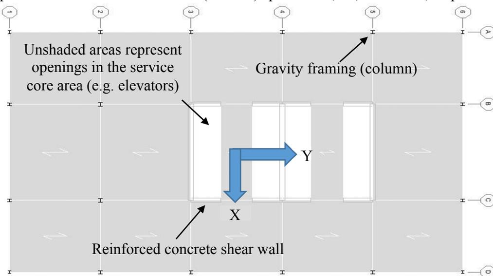
**Figure 1. Typical plan view of building (plan at the 16th story).**
