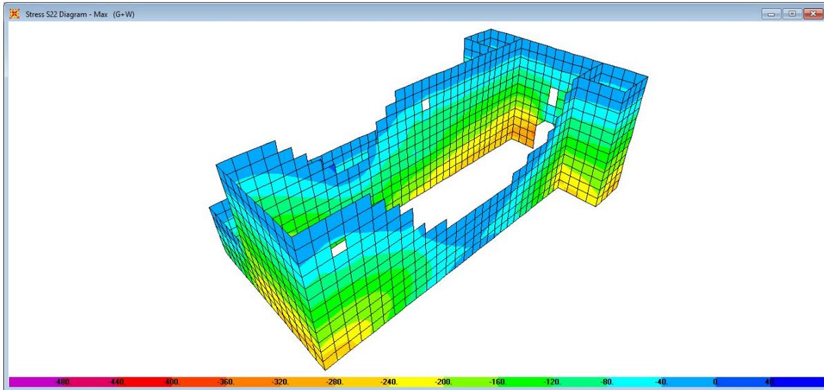
**Figure 7. Stress distribution due to combination of gravity and wind force analysis in the collapsed structure.**
