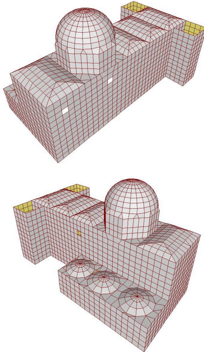
**Figure 6. Finite element model of the reconstructed structure.**
