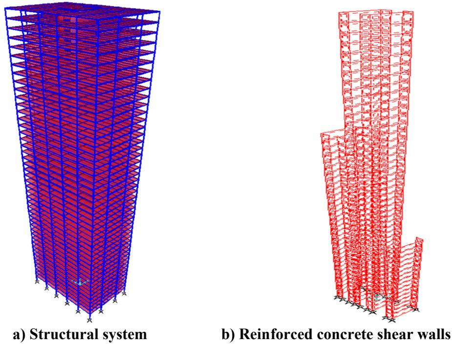
a) Structural system                      b) Reinforced concrete shear walls
