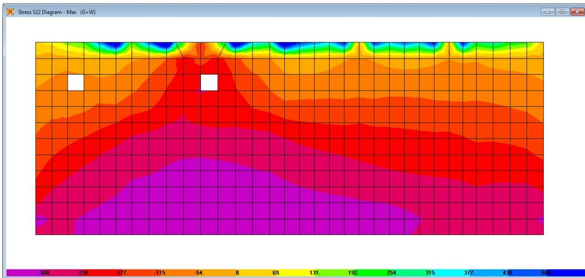
**Figure 10. Compressive stress distribution due to gravity and wind analysis in the repaired structure.**
