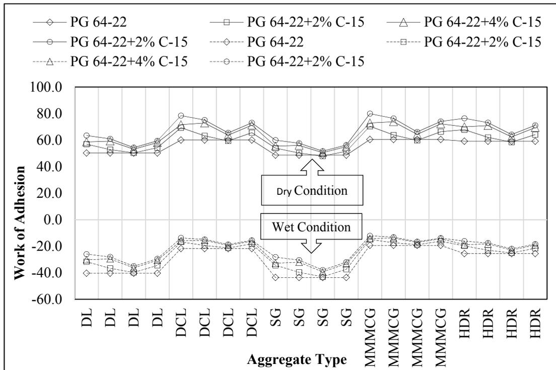
FIG. 5. Work of Adhesion of all Binder-Aggregate Combinations.
