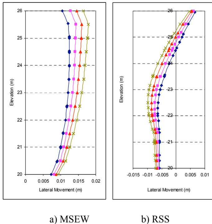
**Figure 6. Lateral movement of slope face subjected to different loading conditions**
