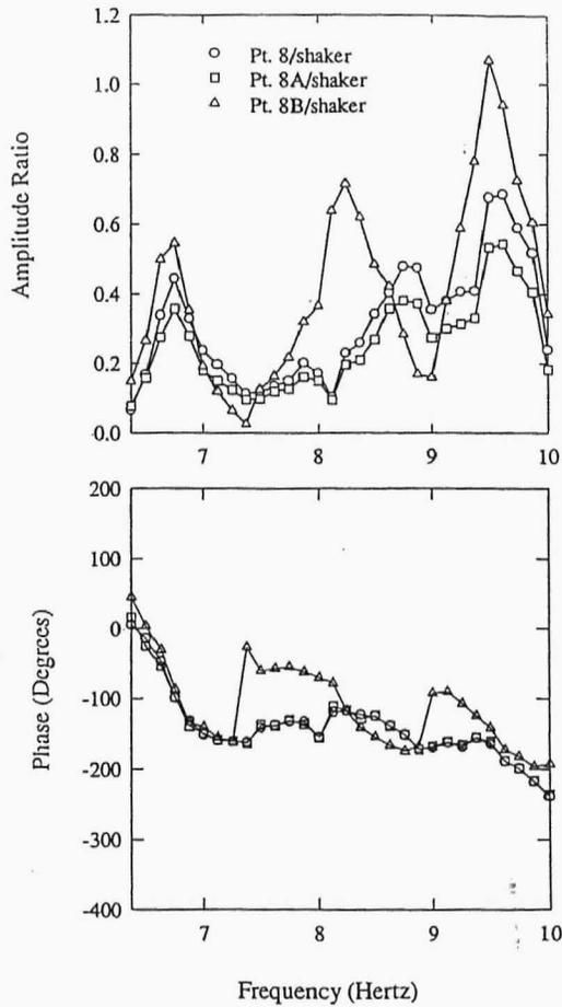
**Figure 9. Typical Acceleration Transfer Function for Points 8, 8A, and 8B (0-10 Hz range)**
