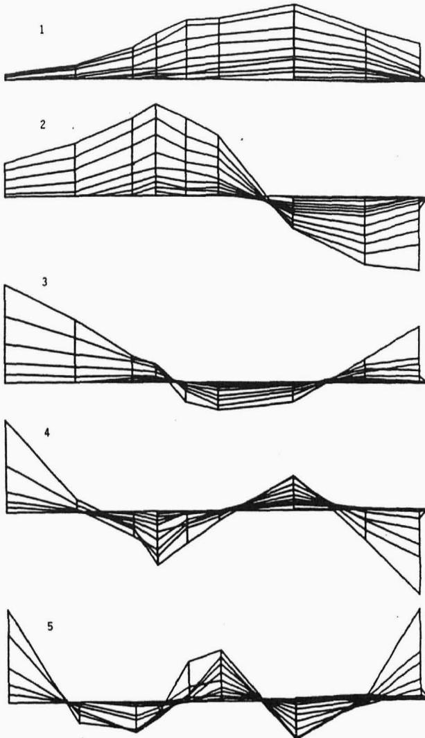
**Figure 4. Mode Shapes of JEC Wall in Plan View**
