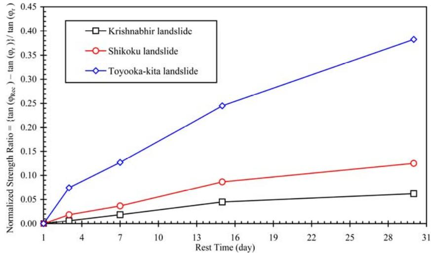
**Fig. 3. Normalized strength ratio versus rest time.**
