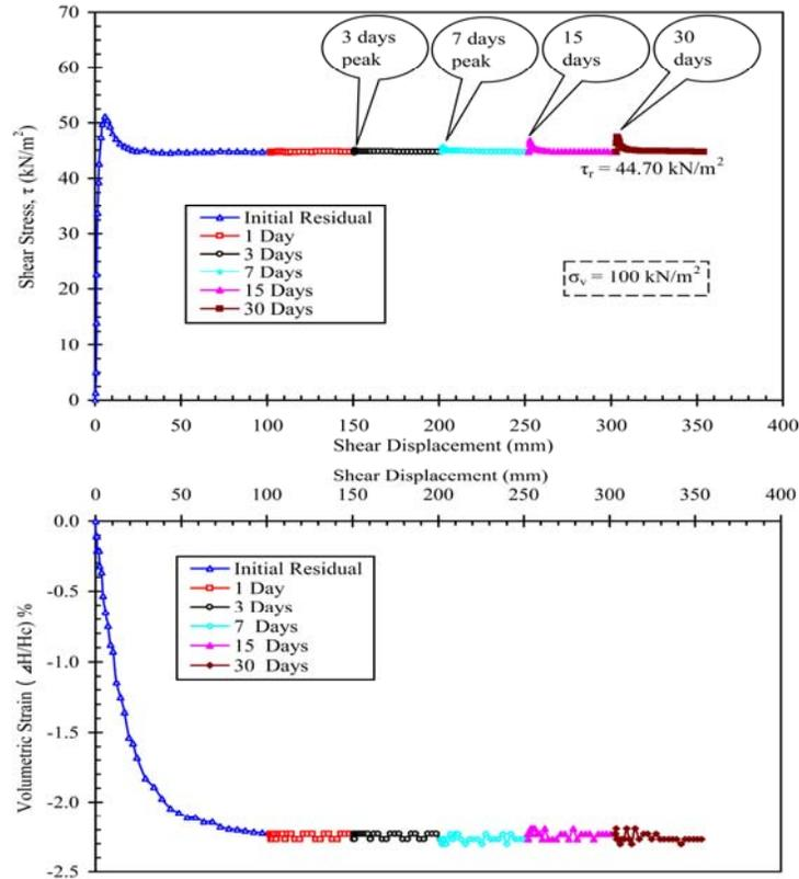
**Fig. 1. Typical results of ring shear tests and strength recovery tests (on Krishnabhir landslide).**
