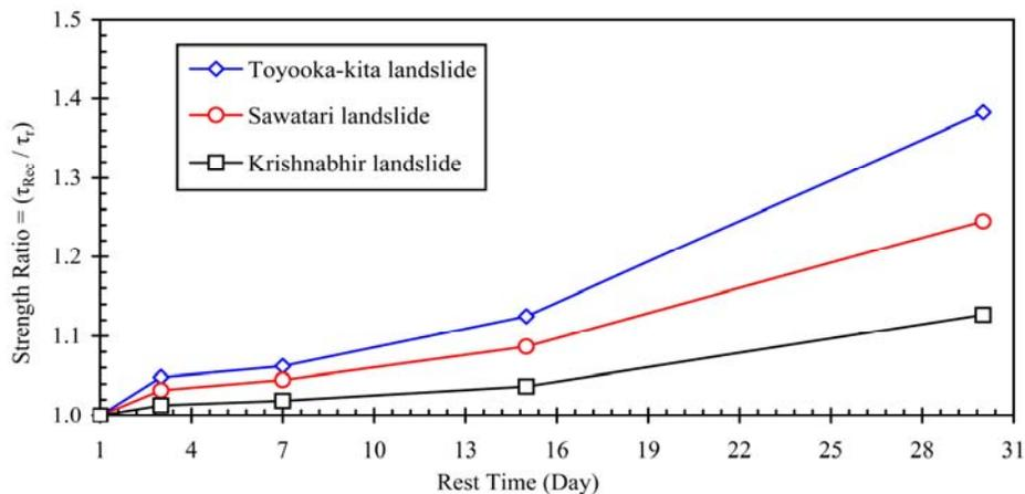
**Fig. 2. Strength ratio versus rest time.**
