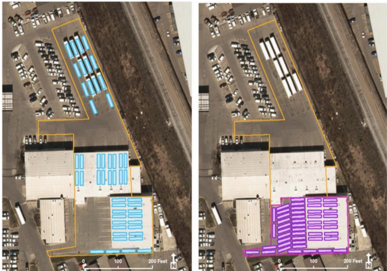
Figures 1 and 2. Example of yard realignment through use of bus automation, with current conditions (left) and potential efficient re-configuration of the same rolling stock (right). (Courtesy of FTA's Strategic Transit Automation Research Plan)
