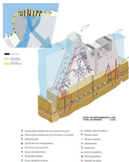
**Figure 2: Dam Key Block - Instruments Location**
