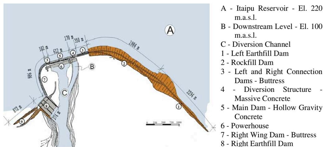
**Figure 1: General Lay-out of Itaipu Dam**
