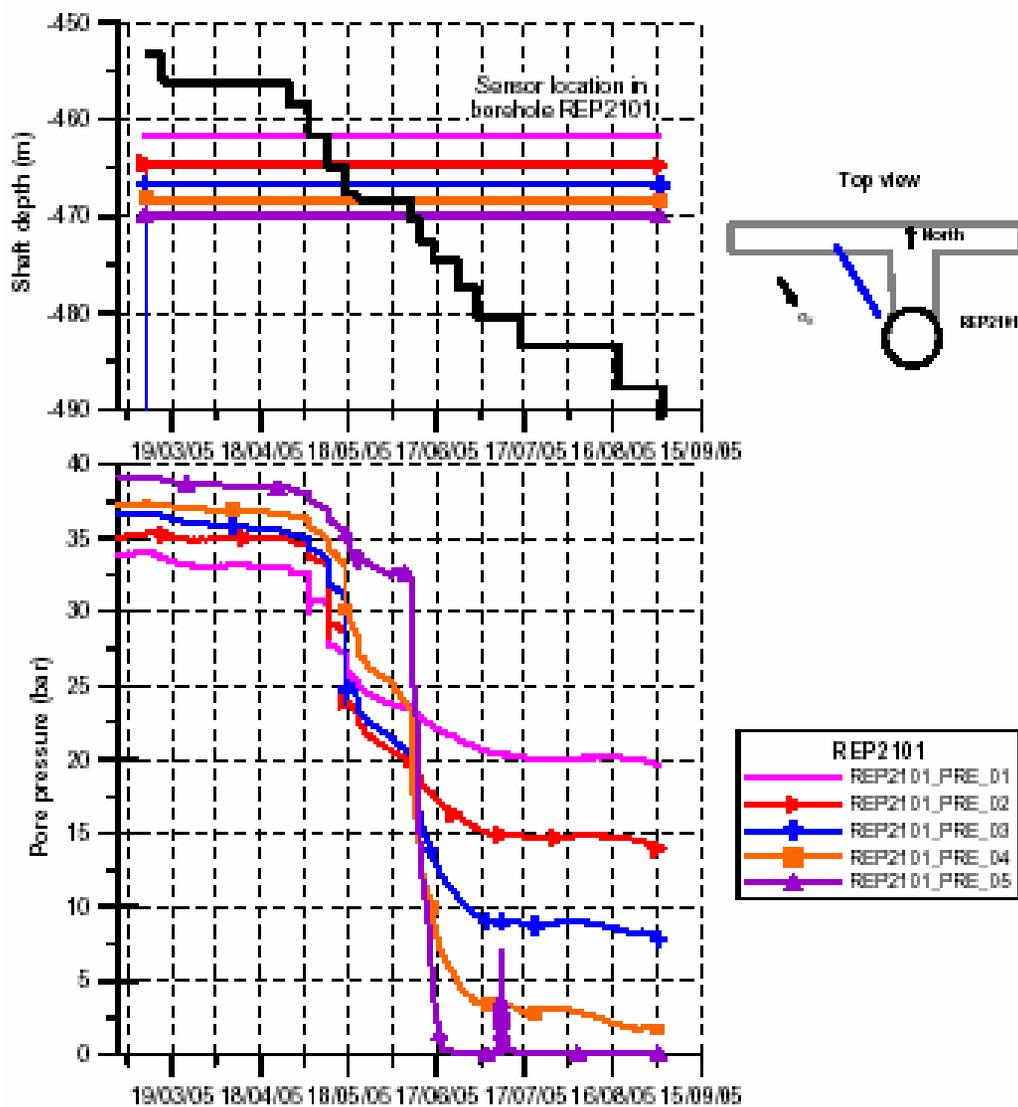
Fig. 5: Evolution of pore pressure in REP2101
