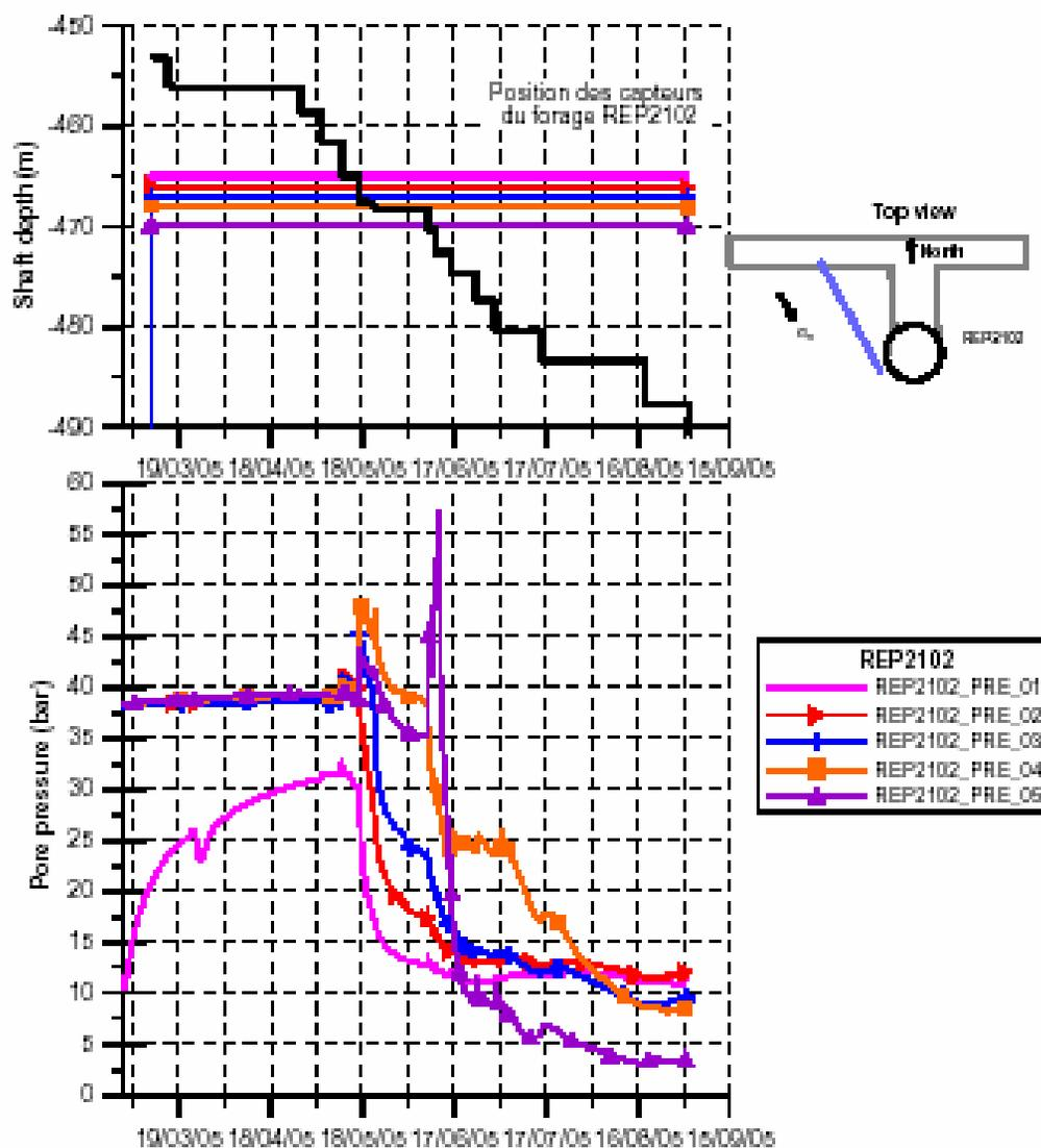
Fig. 6: Evolution of pore pressure in REP2102
