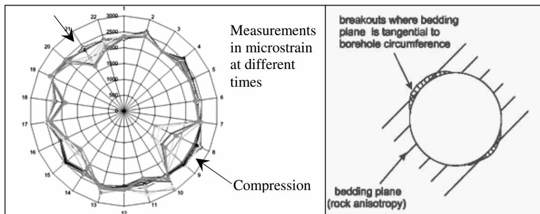
Figure 11: Deformations in the microtunnel measured by the strain gages (left), expected deformations in anisotropic rock (right); source: Mont Terri Consortium.
