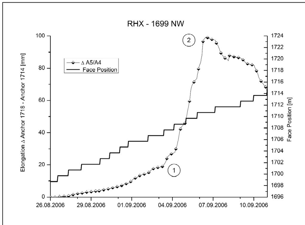
Figure 8 Detail plot: Elongation of two anchoring points of RHX-1699-NW
