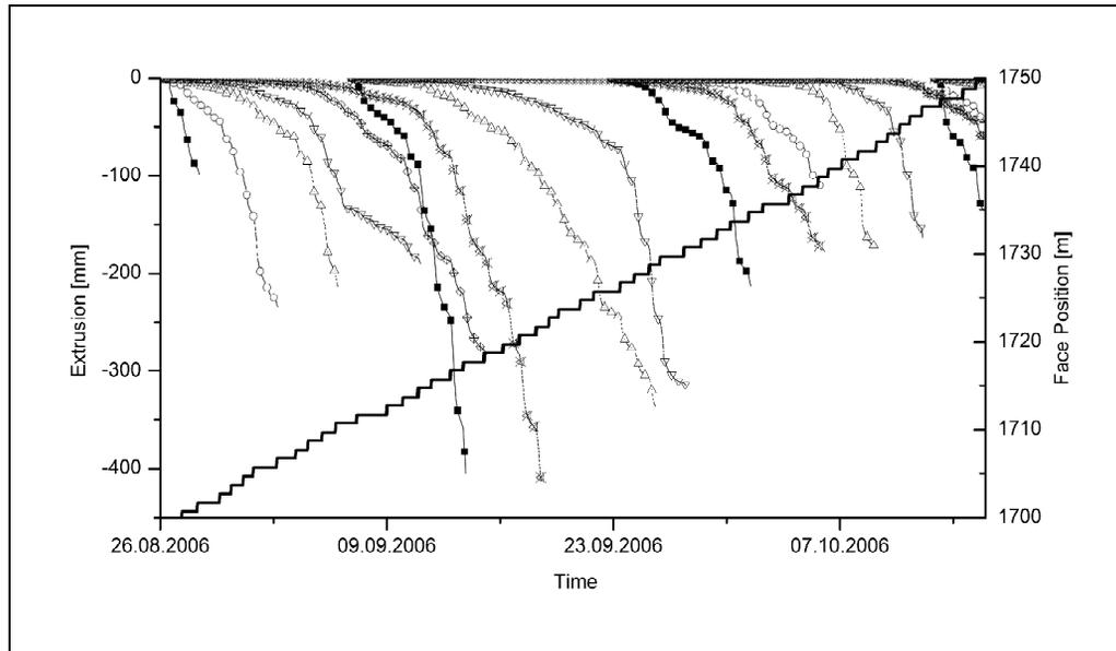
Figure 7 Measurements of overlapping installed RH-Extensometer (RH1699 –RH1747), Sedrun
