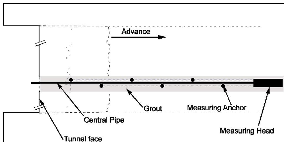
Figure 1 Scheme of a RH Extensometer
