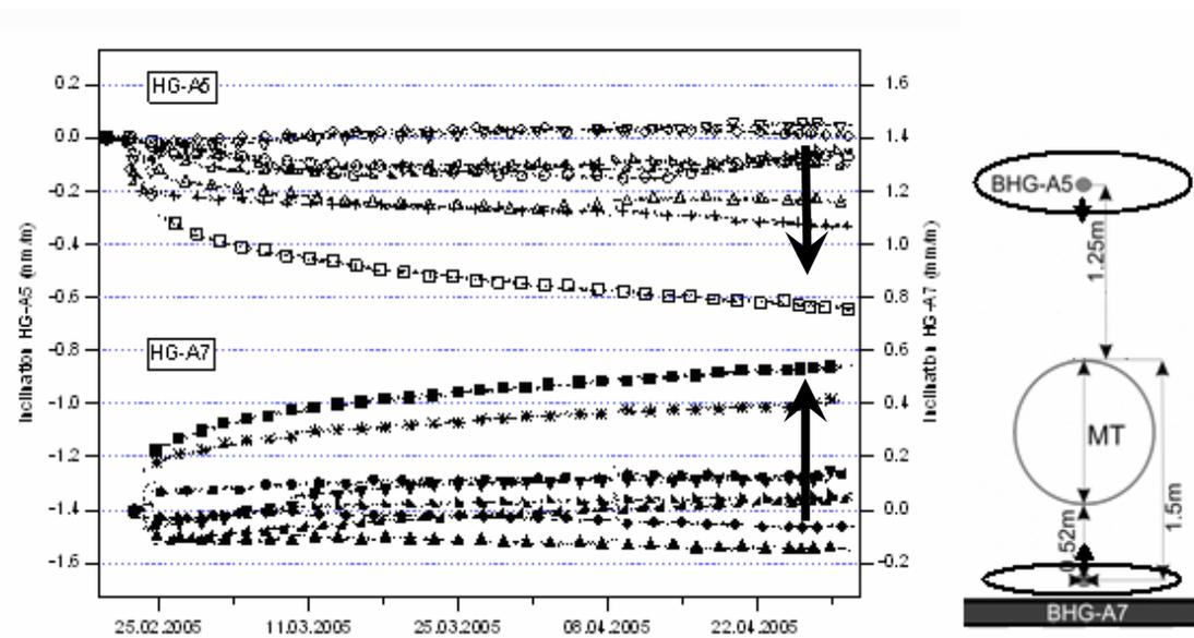
Figure 7: Data plot of the inclinometer chains installed in the boreholes BHG-A5 and BHG-A7 (right side). Location of the axial boreholes BHG-A5 and BHG-A7 in relation to the microtunnel (MT) and the displacement directions (arrows); source: Mont Terri Consortium.
